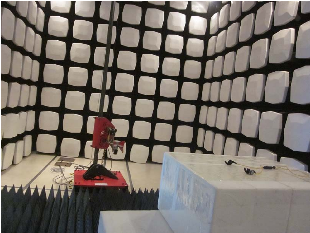
Measurement of Radiated Emission Test Set Up
