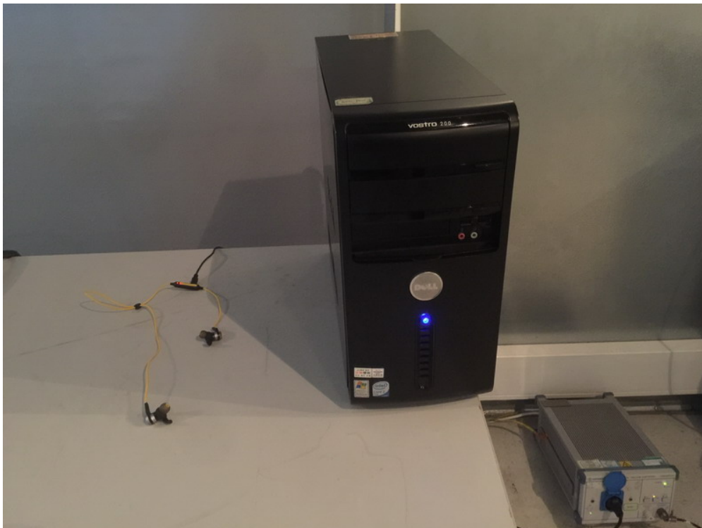
Measurement of Conducted Emission Test Set Up
