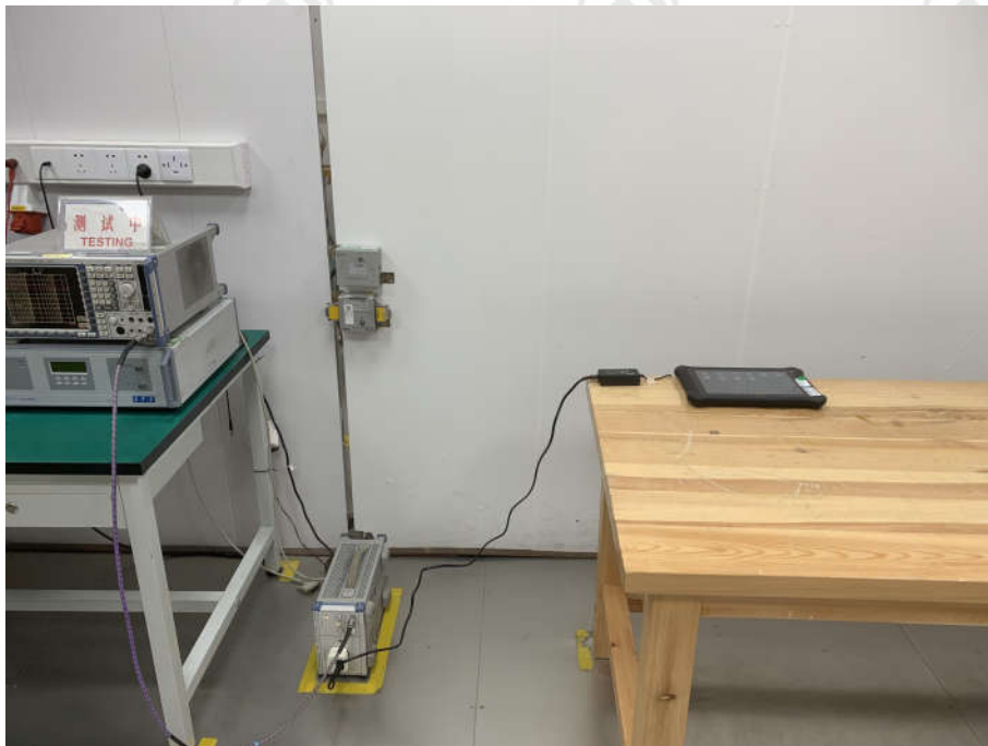
Conducted Emissions Test Setup
