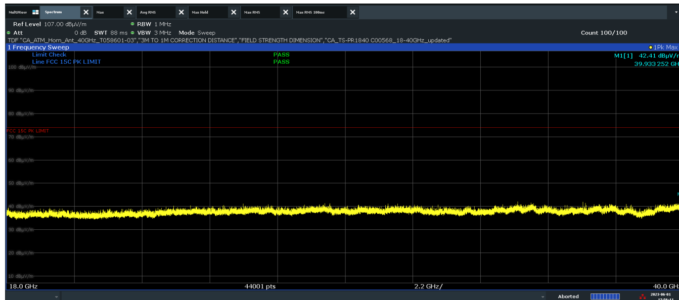
Plot 7-32. Radiated Spurious Emissions above 18GHz (BT GFSK – Ch. 0, Pol H)
