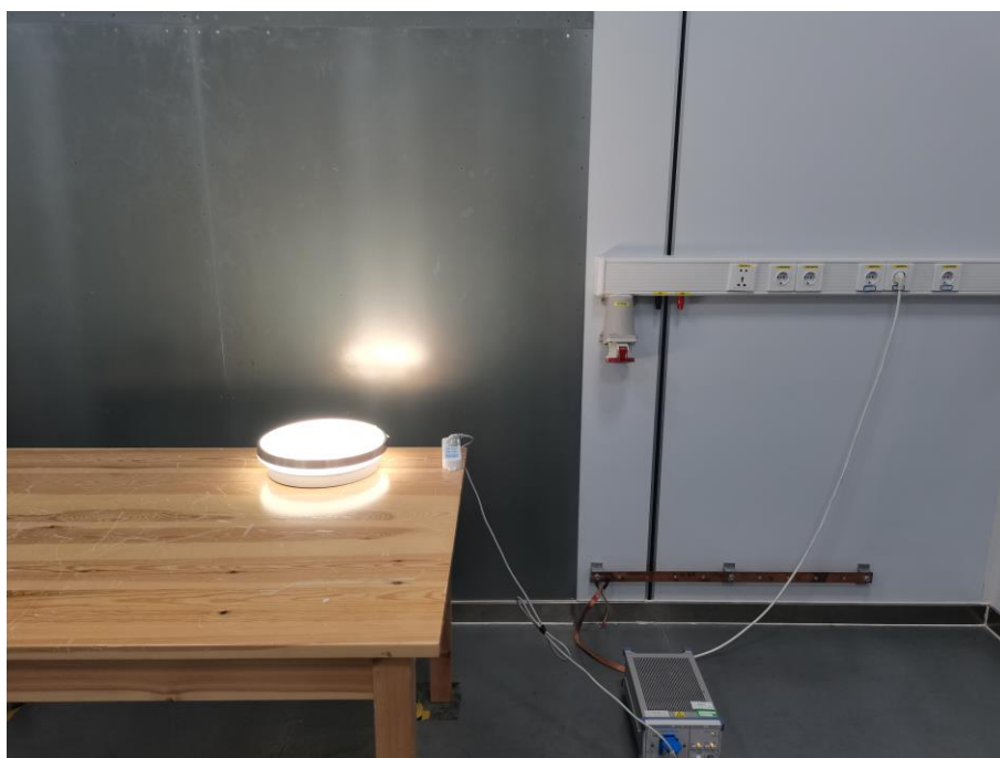
Fig. 4 Power line conducted emission setup photo
