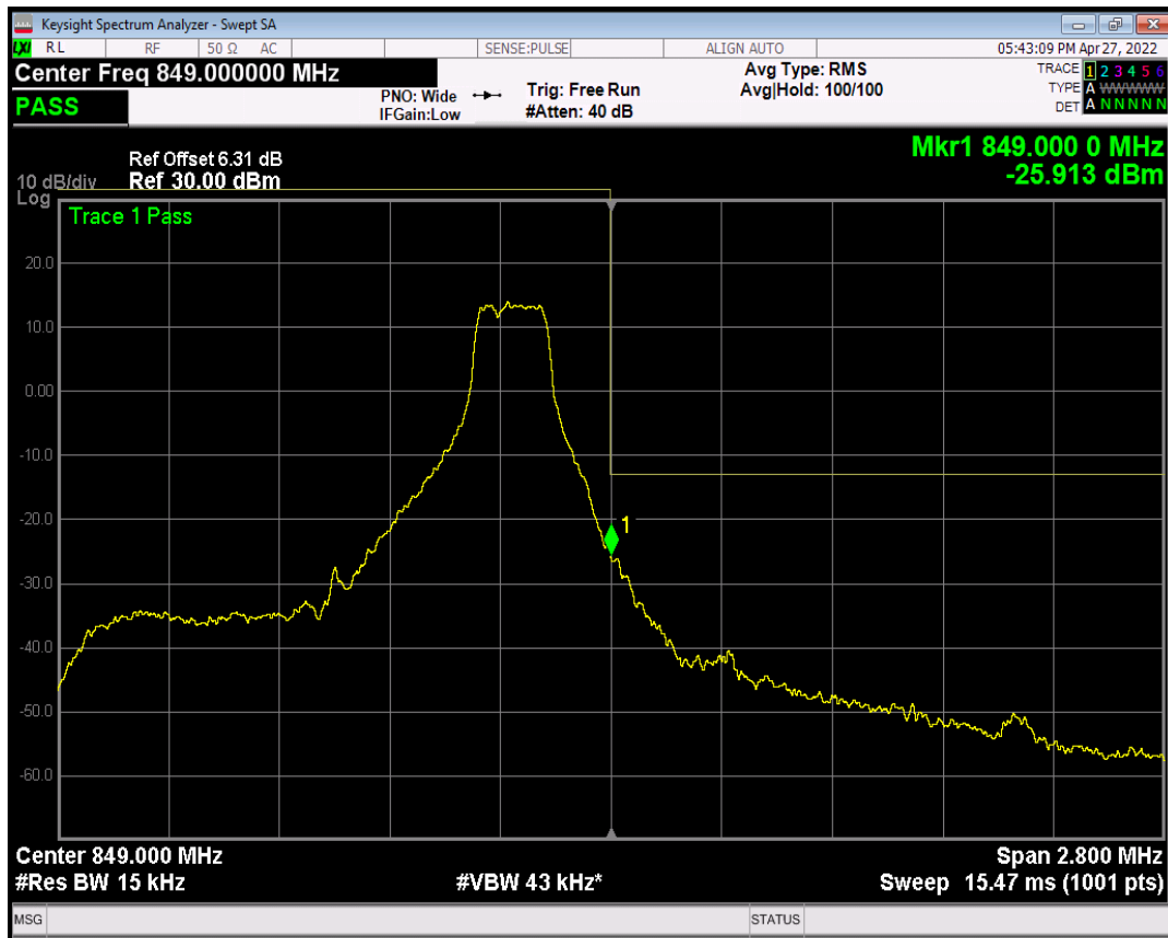
Band5 QPSK BW=1.4MHz Channel=20643 RB Size=6 Position=#0
