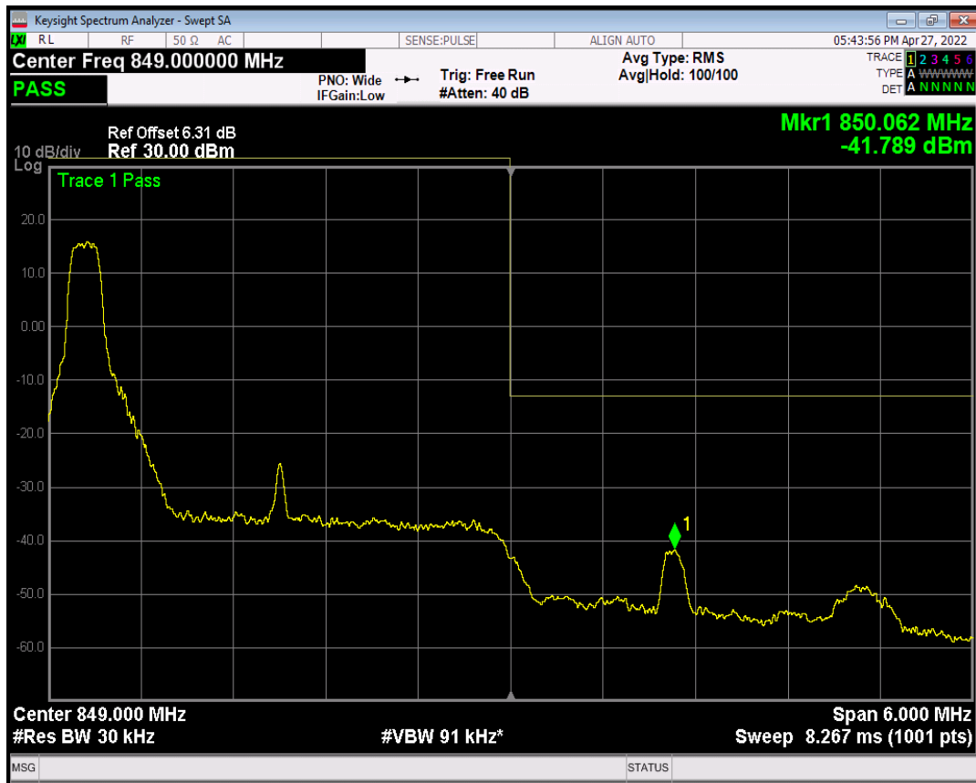
Band5 QAM16 BW=3MHz Channel=20635 RB Size=1 Position=#Max
