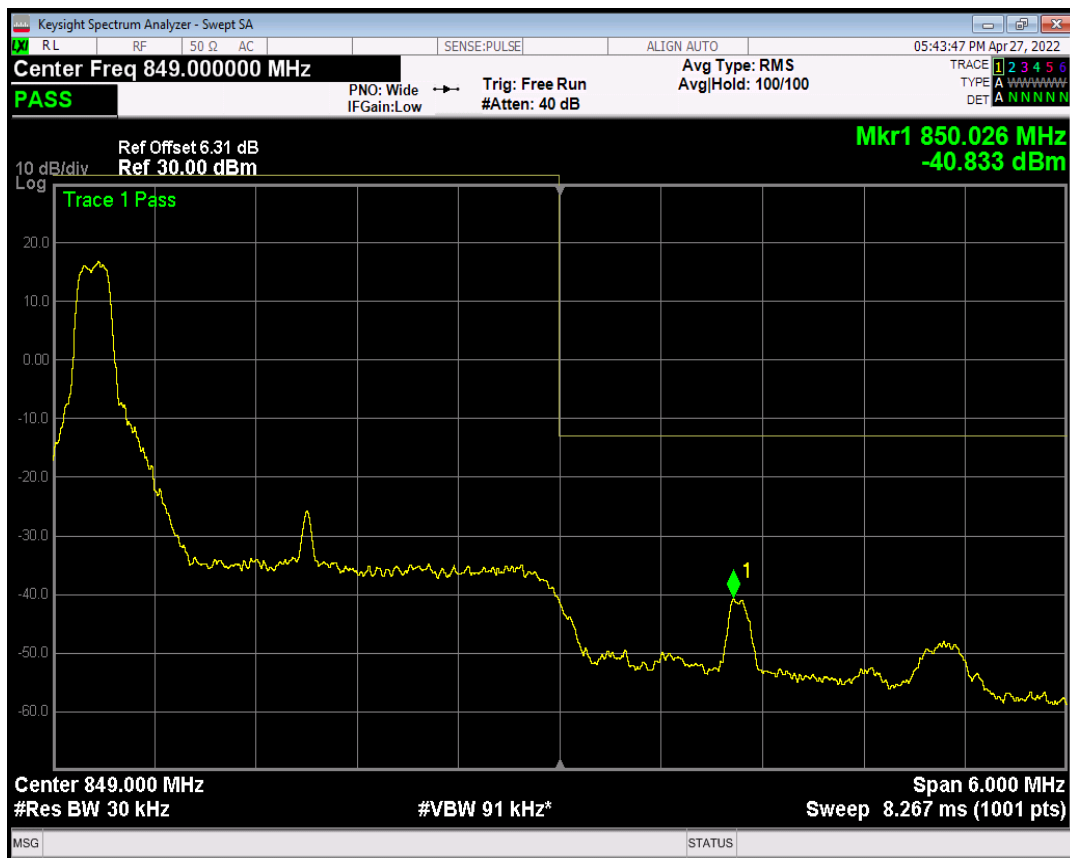
Band5 QPSK BW=3MHz Channel=20635 RB Size=1 Position=#Max
