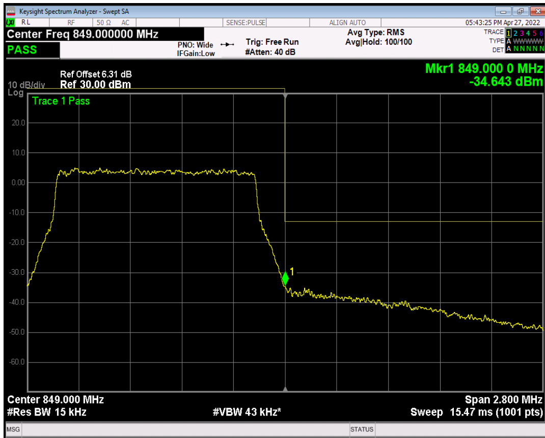
Band5 QPSK BW=3MHz Channel=20415 RB Size=1 Position=#0
