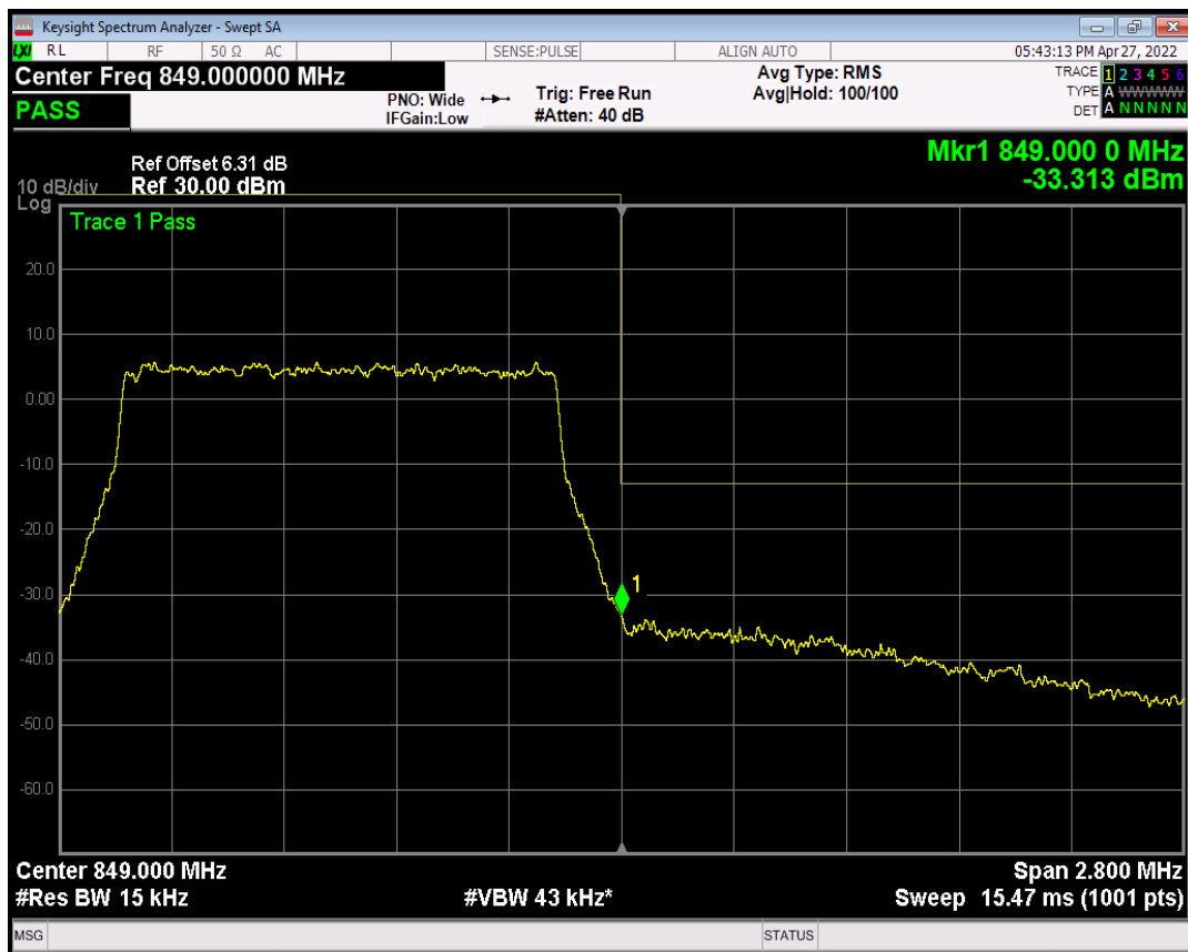
Band5 QAM16 BW=1.4MHz Channel=20643 RB Size=1 Position=#0
