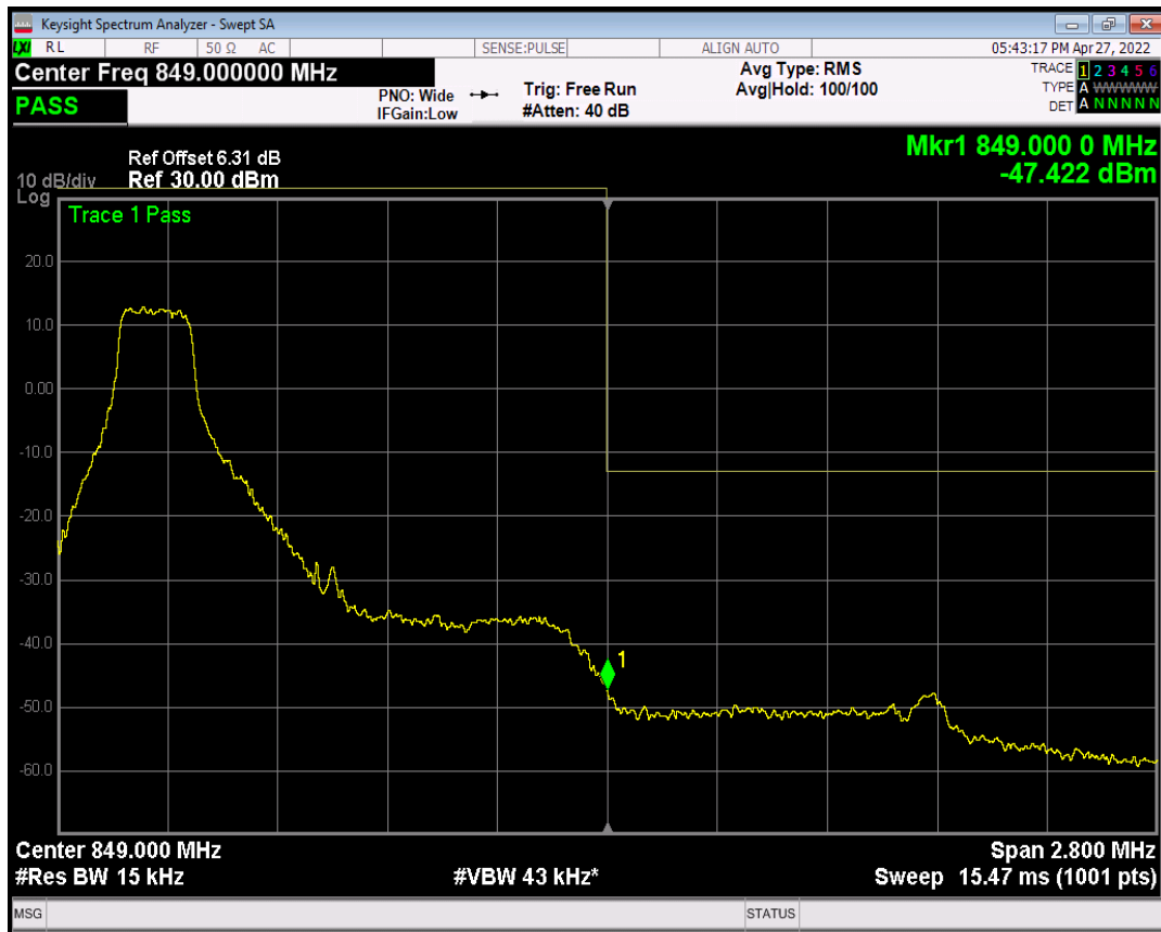
Band5 QAM16 BW=1.4MHz Channel=20643 RB Size=1 Position=#Max
