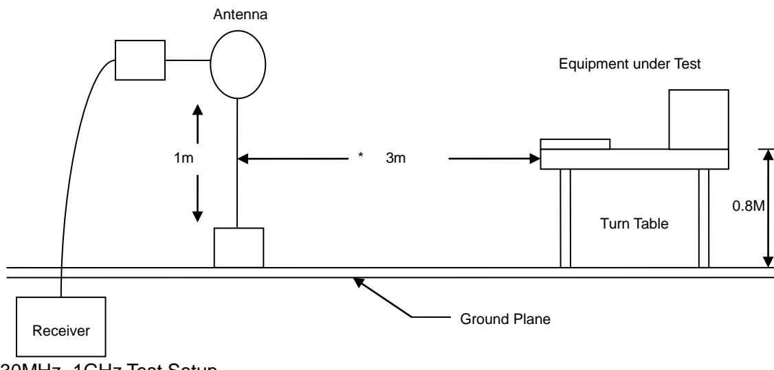
30MHz- 1GHz Test Setup
