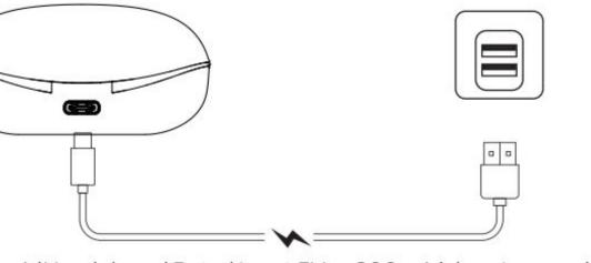
Rated input:5V = 30mA(Headphone)Rated input:5V = 300mA(charging case)
