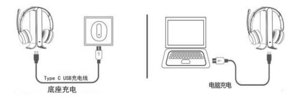
Type-C charging cable / Charging with Base/ Charging with PC
