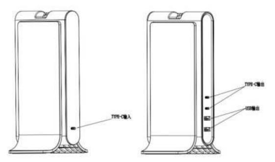
Type-c Input / Type-c Output / USB Output
