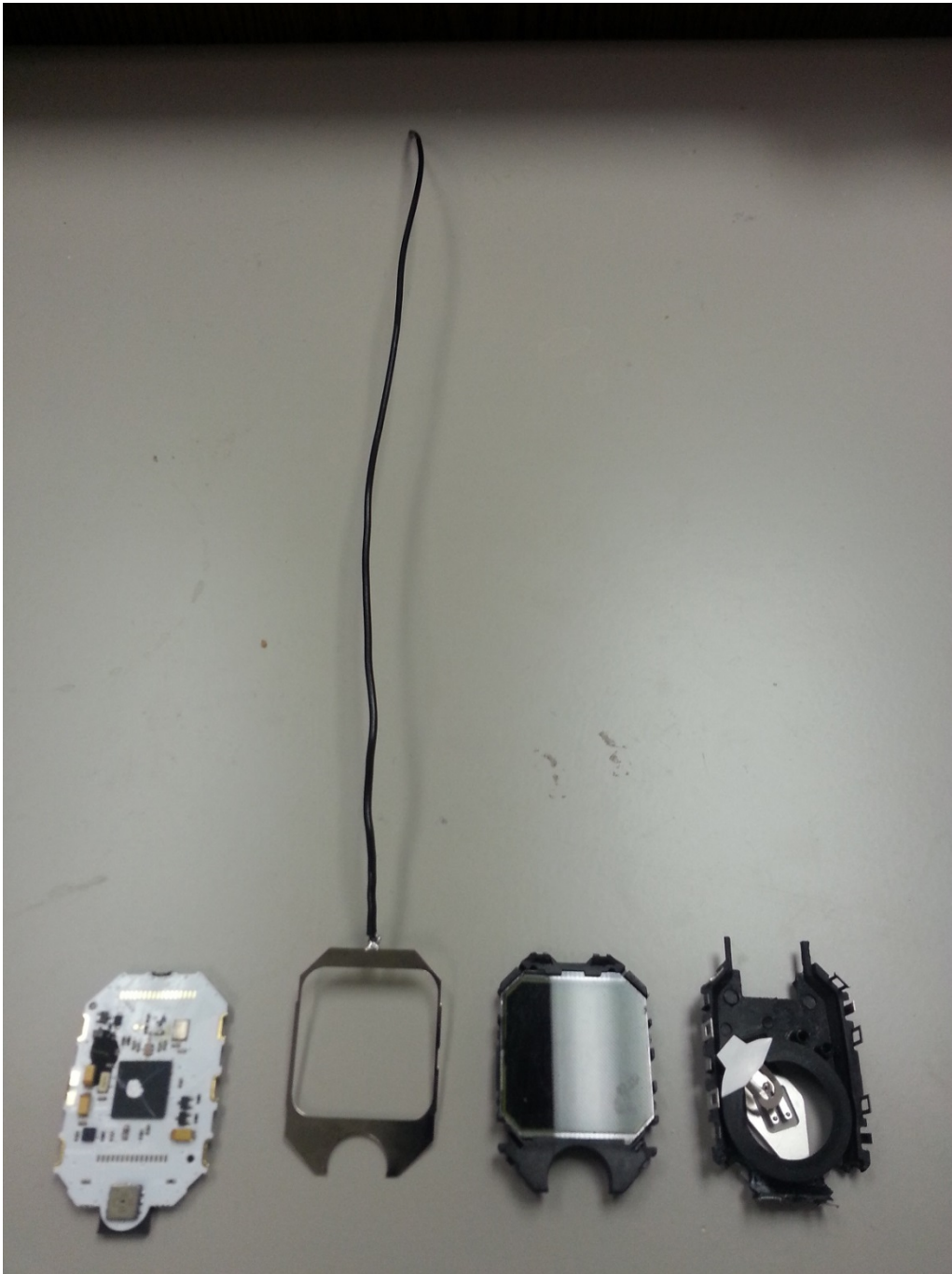
Internal View of Programmer Components (PCB, Antenna, LCD, Battery Holder)
