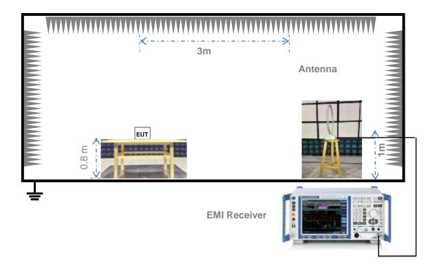
For Radiated Emission Test (Below 30 MHz))
