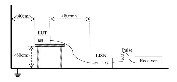
(For Conducted Emission, AC Ports Test)
