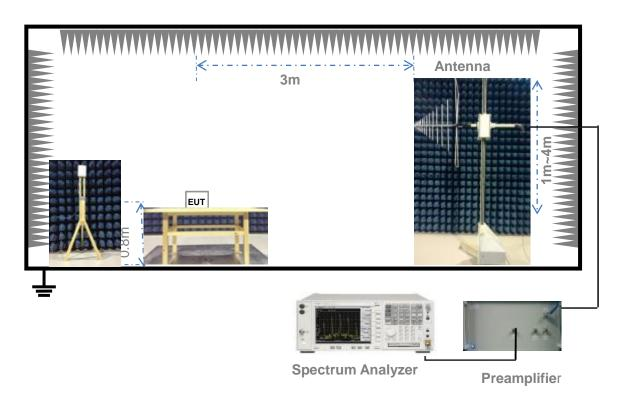
(For Radiated Emission Test (30 MHz-1 GHz))
