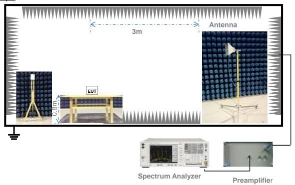
(For Radiated Emission Test (above 1 GHz))
