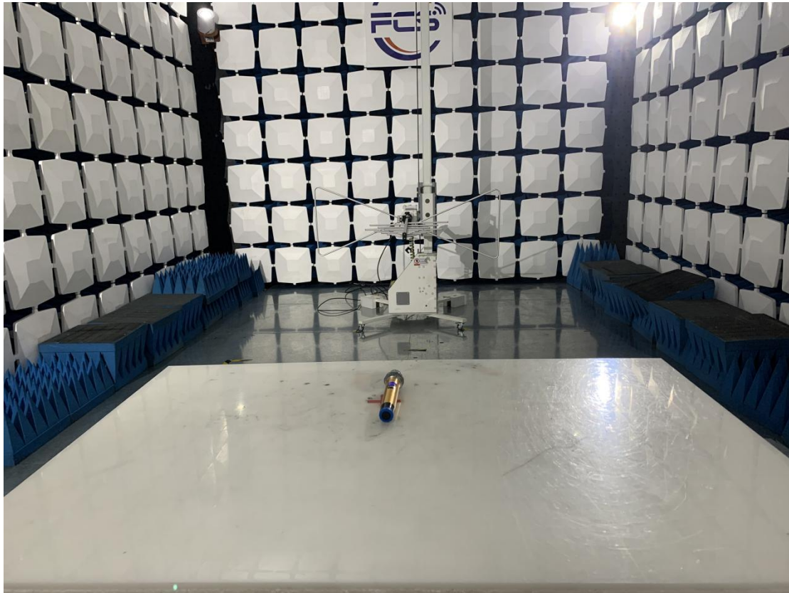
Below 1GHz for radiated emission test setup
