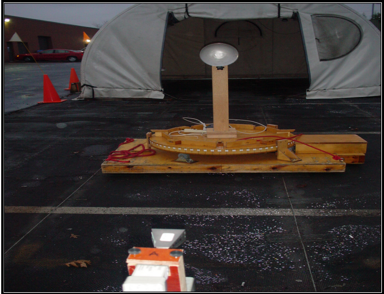
PHOTOGRAPH 3: RADIATED EMISSIONS FRONT VIEW
