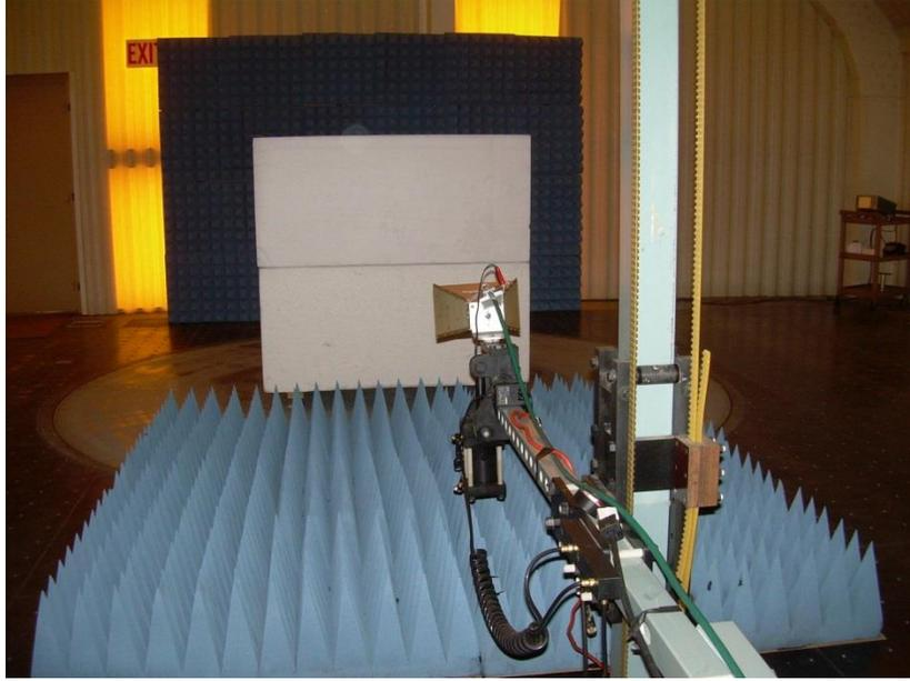
**Photograph 7: Test Setup for Emissions Above 1000 MHz**
