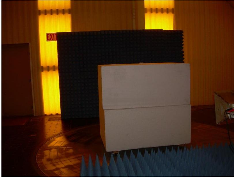
**Photograph 3 – Front View Radiated Emissions – Above 1000 MHz Configuration**
