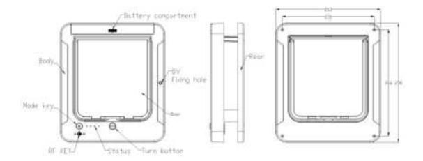
1. The cat door has four access control modes, namely, no entry and no exit, only entry and no exit, only exit and no entry, and entry and exit.
