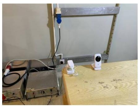
Radiated Emissions (30MHz-1GHz) Test Setup
