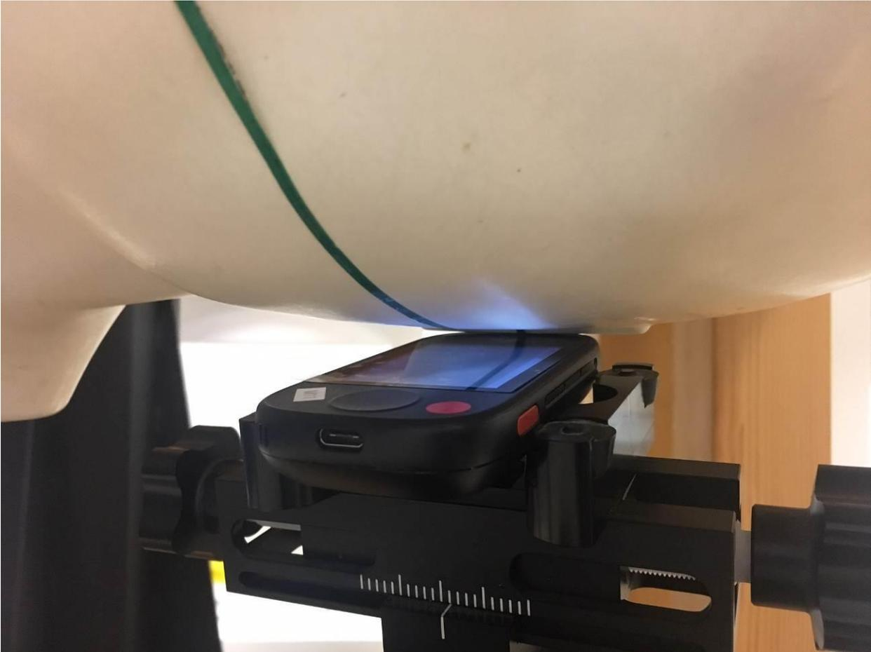
*Figure 3: Test Setup (Right Ear- Cheek Touch)*
