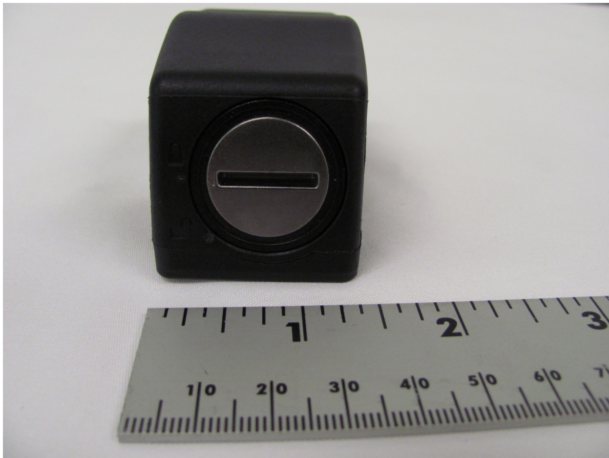
Figure 6. Battery side with Battery Pack Installed
