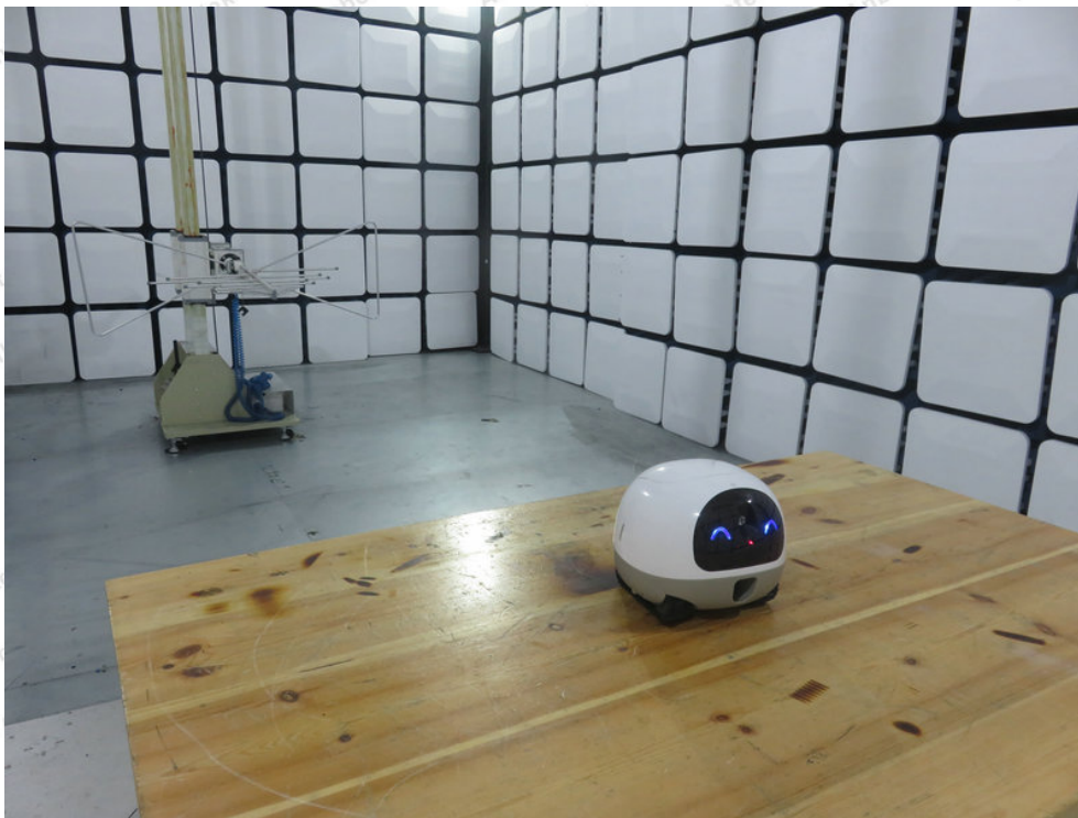
Photo of Radiation Emission Test
