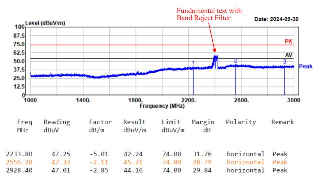
Project No.: 2407X56114E-RF Test Mode: 11g-2412 EUT Model: YS-R1PLUS Test distance: 3m
