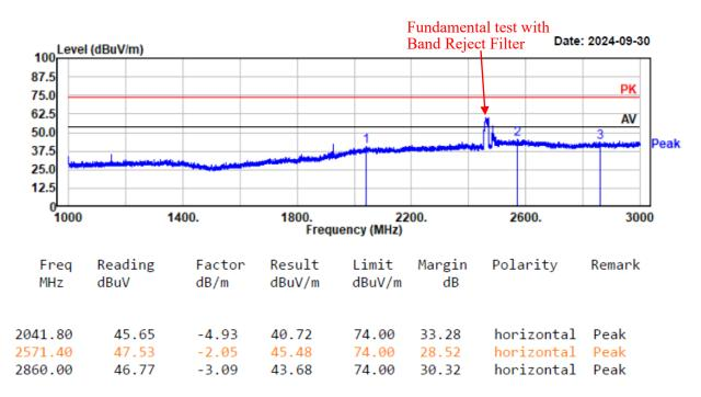
Project No.: 2407X56114E-RF Test Mode: 11n20-2462 EUT Model: YS-R1PLUS Test distance: 3m
