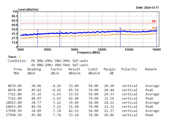
Project No.: 2407X56114E-RF Test Mode: 11n20-2462 EUT Model: YS-R1PLUS Test distance: 3m
