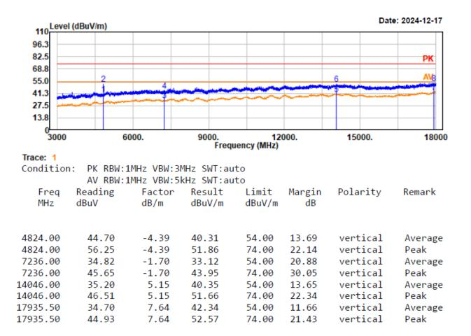
Project No.: 2407X56114E-RF Test Mode: 11b-2437 EUT Model: YS-R1PLUS Test distance: 3m
