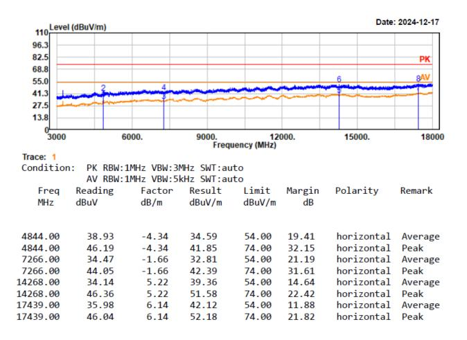
Project No.: 2407X56114E-RF Test Mode: 11n40-2422 EUT Model: YS-R1PLUS Test distance: 3m
