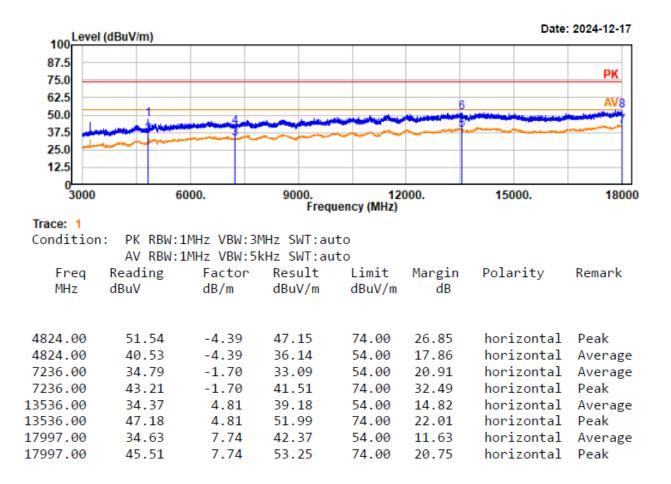
Project No.: 2407X56114E-RF Test Mode: 11n20-2412 EUT Model: YS-R1PLUS Test distance: 3m
