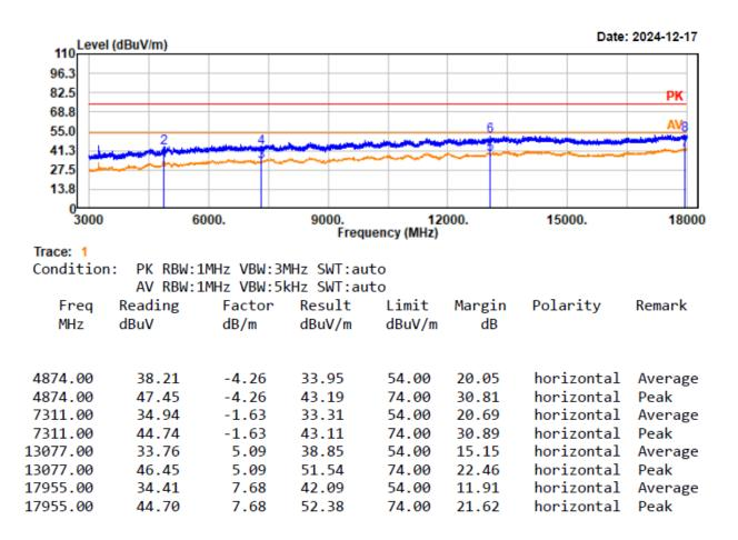
Project No.: 2407X56114E-RF Test Mode: 11n40-2437 EUT Model: YS-R1PLUS Test distance: 3m
