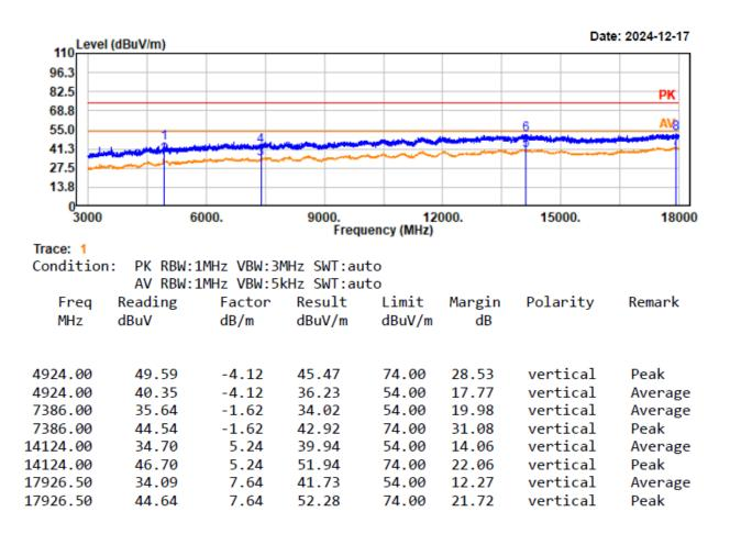
Project No.: 2407X56114E-RF Test Mode: 11n20-2412 EUT Model: YS-R1PLUS Test distance: 3m
