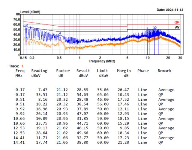
Project No.: 2407X56114E-RF Test Mode: 11B 2437 EUT Model: YS-R1PLUS Temp/Humi/ATM: 21.4°C/56%/100.1kPa Tested by: Spike Gao Power Source: AC 120V/60Hz
