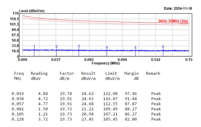
Project No.: 2407X56114E-RF Test Mode: 11B 2437 EUT Model: YS-R1PLUS Test distance: 3m Temp/Humi/ATM: 21.5℃/48%/100.3kPa Tested by: Wlif Wu Power Source: AC120V/60Hz
