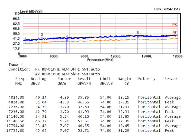
Project No.: 2407X56114E-RF Test Mode: 11g-2412 EUT Model: YS-R1PLUS Test distance: 3m
