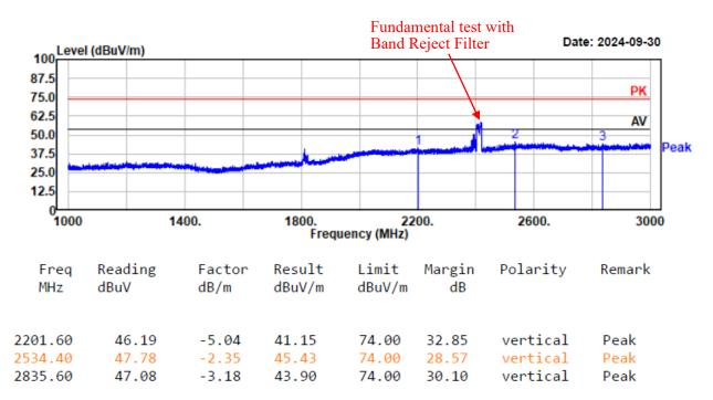
Project No.: 2407X56114E-RF Test Mode: 11g-2437 EUT Model: YS-R1PLUS Test distance: 3m
