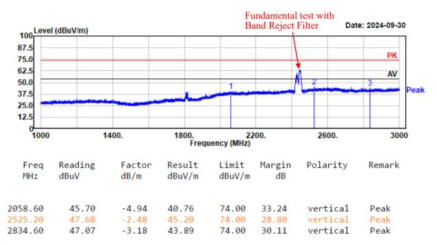
Project No.: 2407X56114E-RF Test Mode: 11n40-2452 EUT Model: YS-R1PLUS Test distance: 3m
