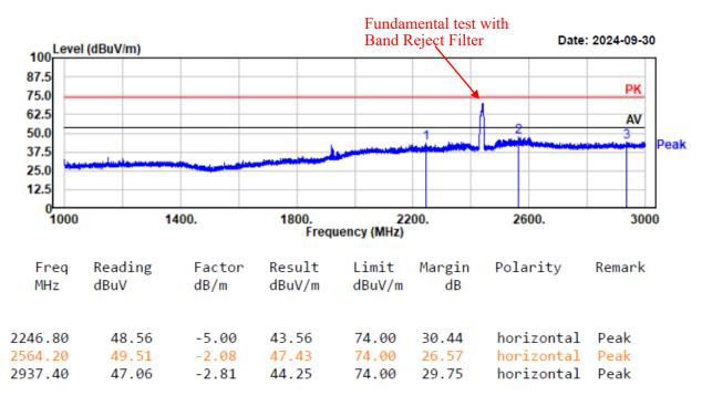
Project No.: 2407X56114E-RF Test Mode: 11b-2437 EUT Model: YS-R1PLUS Test distance: 3m
