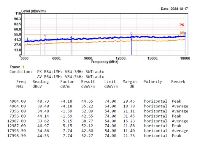
Project No.: 2407X56114E-RF Test Mode: 11n40-2452 EUT Model: YS-R1PLUS Test distance: 3m
