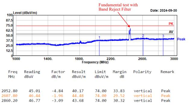
Project No.: 2407X56114E-RF Test Mode: 11g-2462 EUT Model: YS-R1PLUS Test distance: 3m
