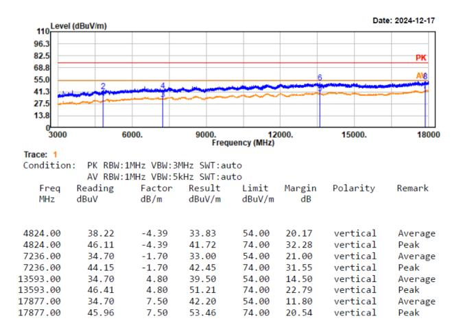
Project No.: 2407X56114E-RF Test Mode: 11n20-2437 EUT Model: YS-R1PLUS Test distance: 3m Temp/Humi/ATM: 21.5℃/46%/100.1kPa Tested by: Wlif Wu Power Source: AC120V/60Hz
