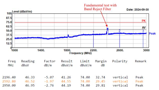
Project No.: 2407X56114E-RF Test Mode: 11n20-2437 EUT Model: YS-R1PLUS Test distance: 3m
