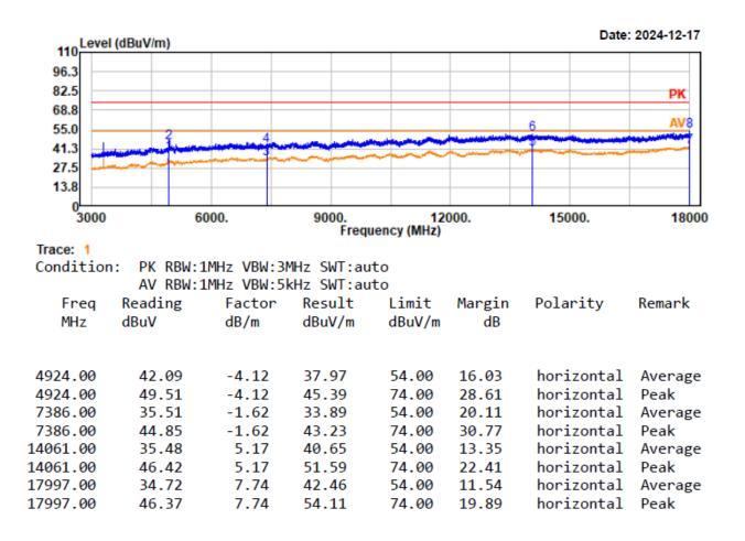
Project No.: 2407X56114E-RF Test Mode: 11g-2462 EUT Model: YS-R1PLUS Test distance: 3m
