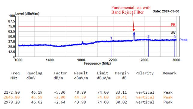
Project No.: 2407X56114E-RF Test Mode: 11n40-2422 EUT Model: YS-R1PLUS Test distance: 3m
