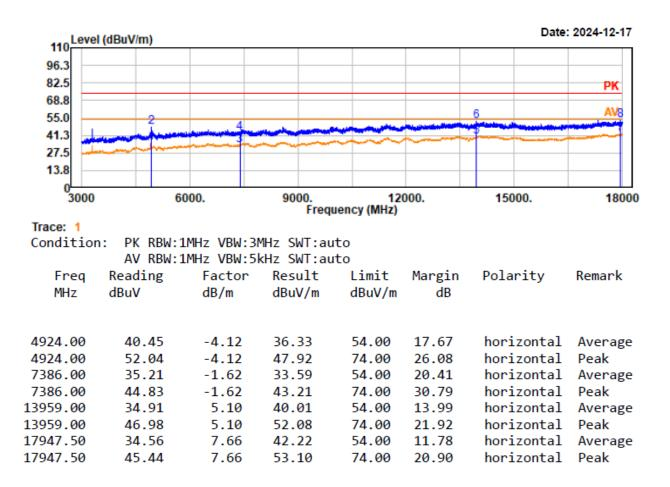
Project No.: 2407X56114E-RF Test Mode: 11n20-2462 EUT Model: YS-R1PLUS Test distance: 3m
