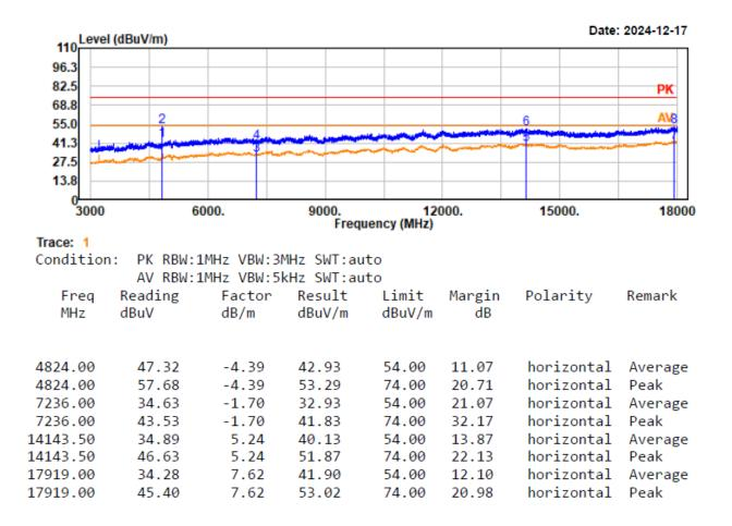
Project No.: 2407X56114E-RF Test Mode: 11b-2412 EUT Model: YS-R1PLUS Test distance: 3m
