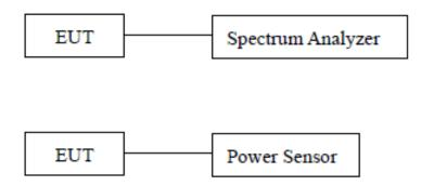
Note: The cable assembly insertion loss of 0.5dB was entered as an offset in the spectrum analyzer/power sensor.(Actual cable loss was unavailable at the time of testing, therefore loss of 0.5dB was assumed as worst case.) This was later verified to be true by laboratory.
