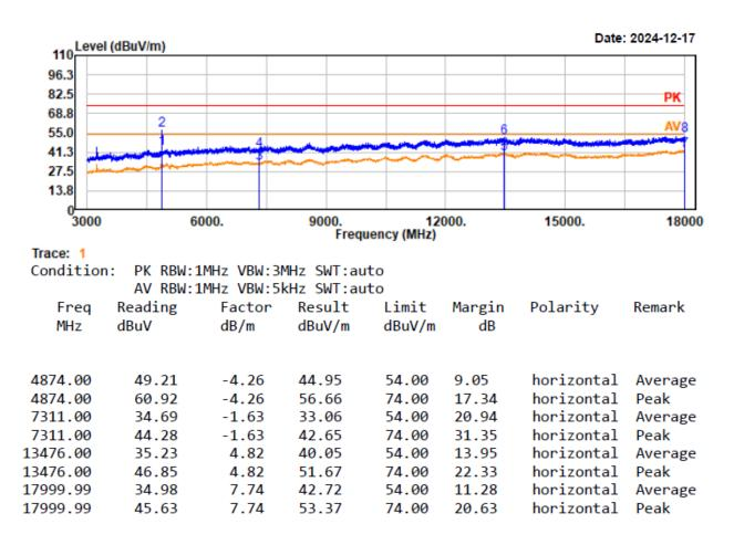
Project No.: 2407X56114E-RF Test Mode: 11b-2437 EUT Model: YS-R1PLUS Test distance: 3m
