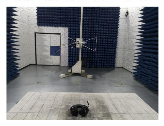
RADIATED EMISSION TEST SETUP ABOVE 1GHZ
