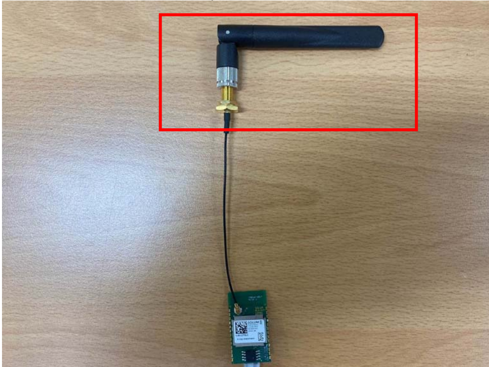
Reverse polarity type antenna
