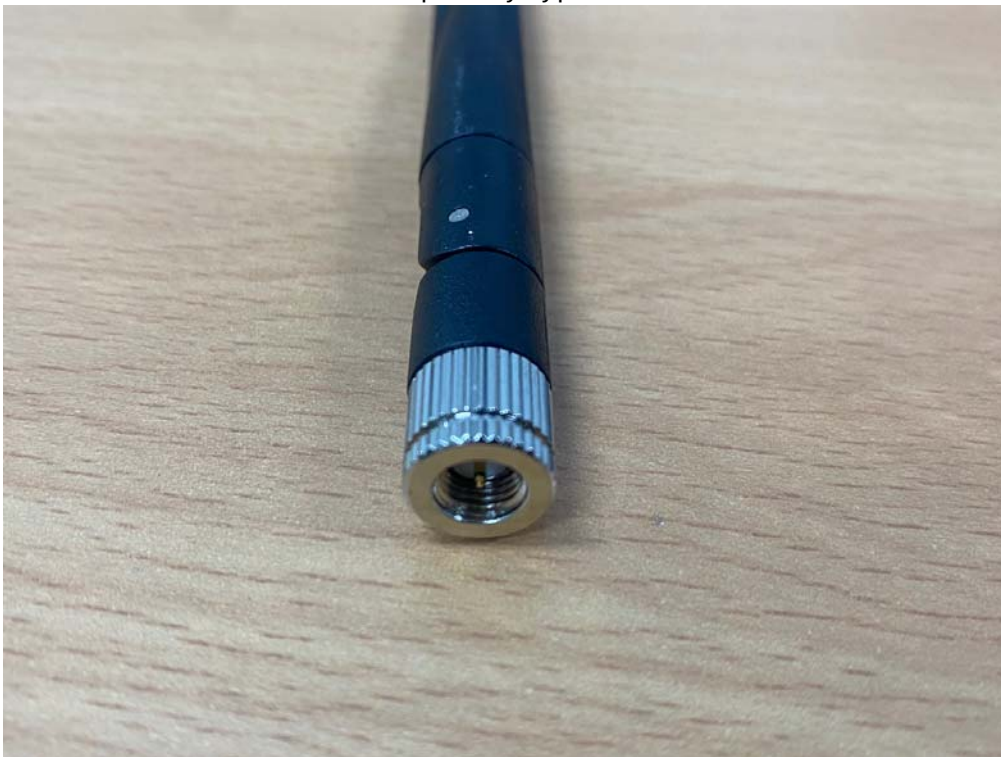
Reverse polarity type antenna
