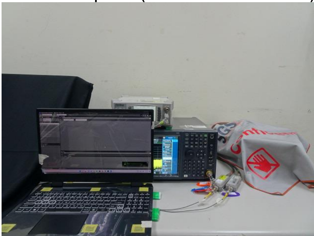
Conducted Setup Photo (Measurement at Antenna Port)
