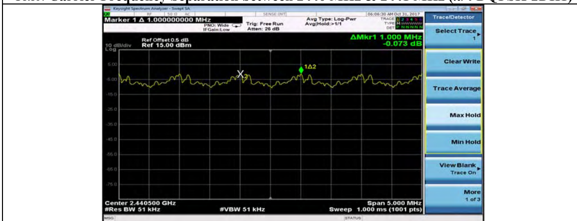
Title: Carrier Frequency Separation between 2440 MHz & 2441 MHz (8-DPSK-3DH1)
