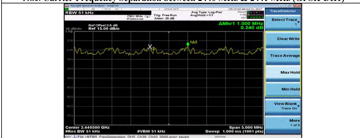
Title: Carrier Frequency Separation between 2440 MHz & 2441 MHz ( \pi/4 DQPSK-2DH1)
