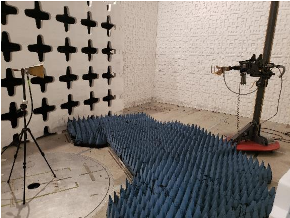
Figure 9. Substitution Test Setup, Above 1 GHz
