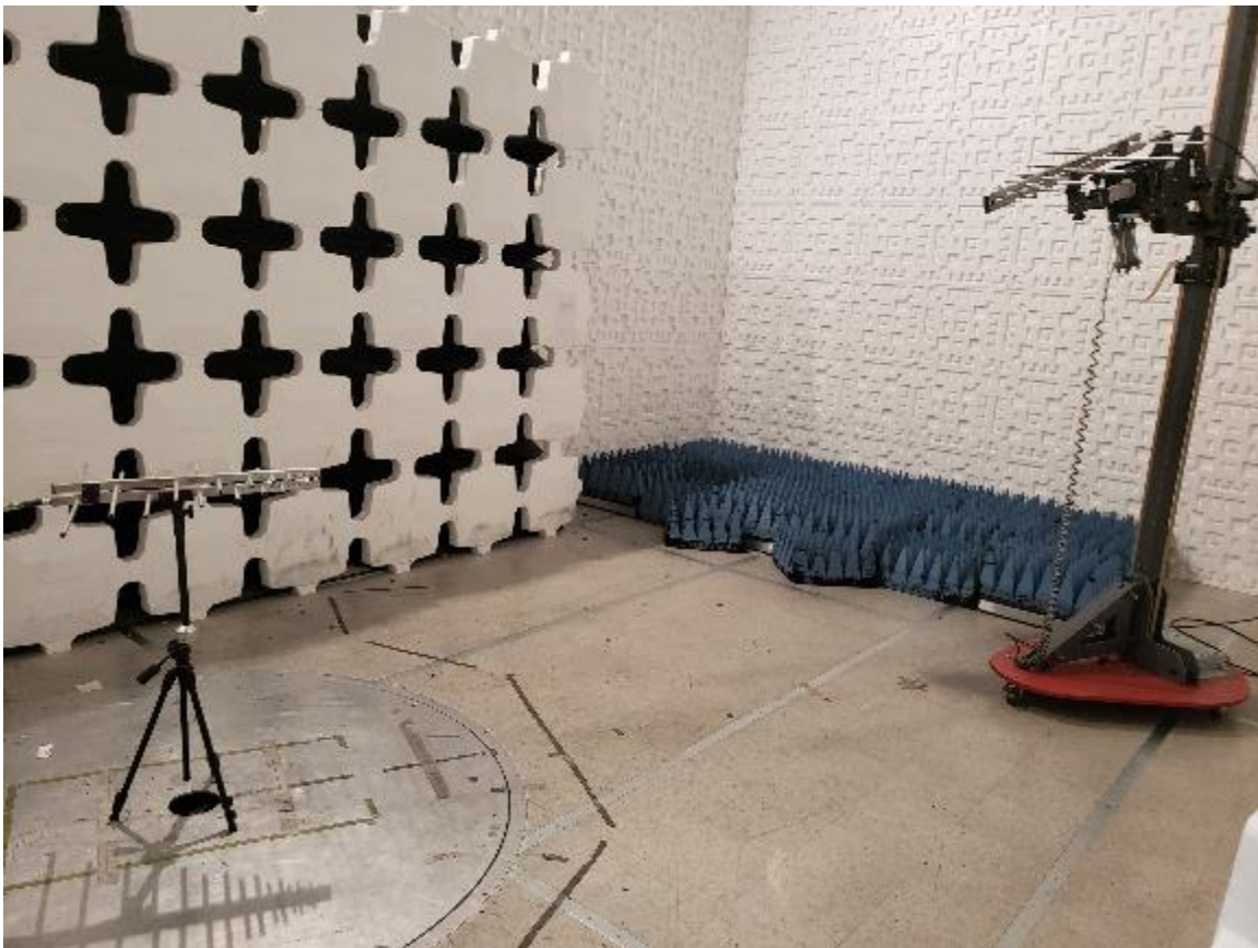
Figure 8. Substitution Test Setup, 200 MHz to 1 GHz
