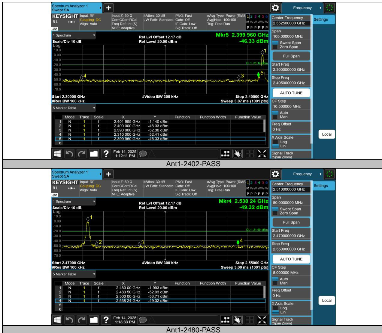
**TEST REPORT****Conducted Spurious Emission****Test Result**
