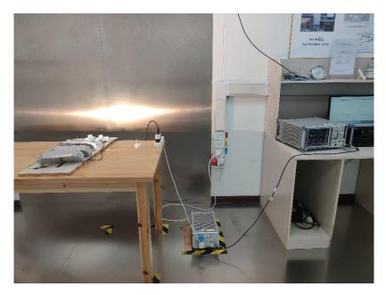
Radiated Emissions From 30MHz-1000MHz
