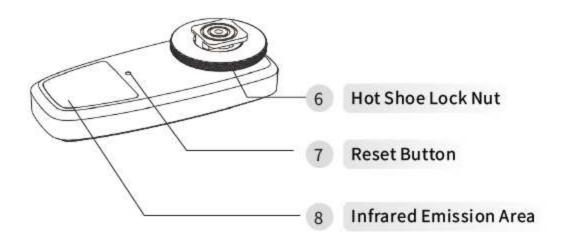
Do not block the infrared emission area during use! The delivered USB cable is for time lapse trigger charging only!
