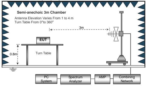
(C) Radiated Emission Test-Up Frequency Above 1GHz
