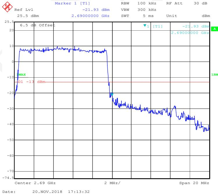
**16-QAM (15 MHz, FULL RB) - Left Band Edge**
