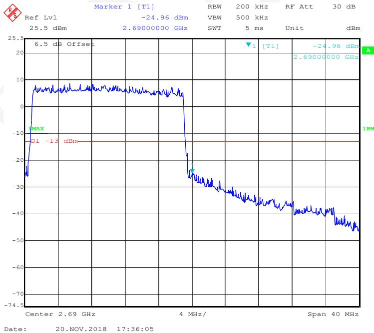
**16-QAM (5MHz, FULL RB) - Left Band Edge**
