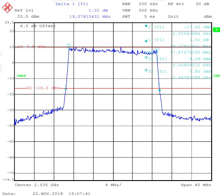
**16-QAM (5 MHz) - Middle channel**
