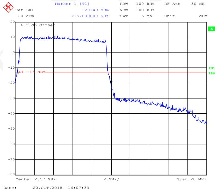
**QPSK (15 MHz, FULL RB) - Left Band Edge**
