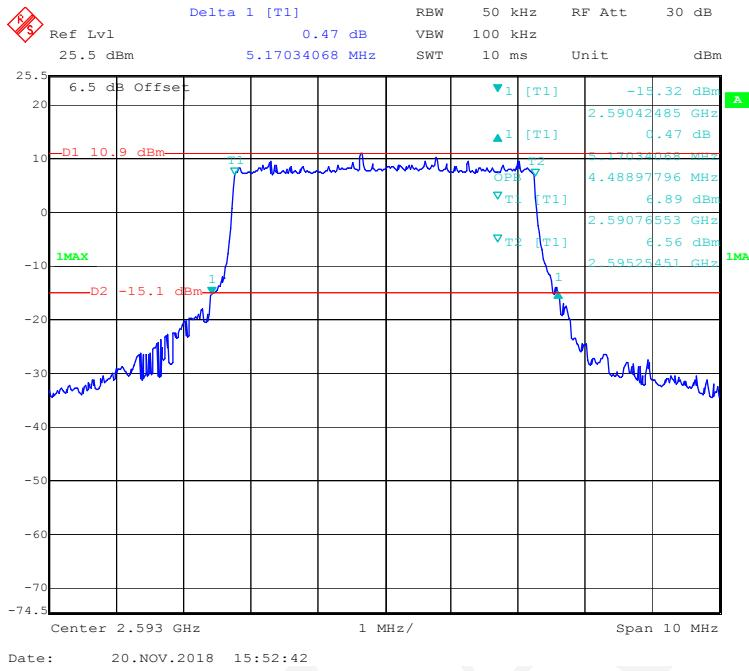
**16-QAM (10 MHz) - Middle channel**
