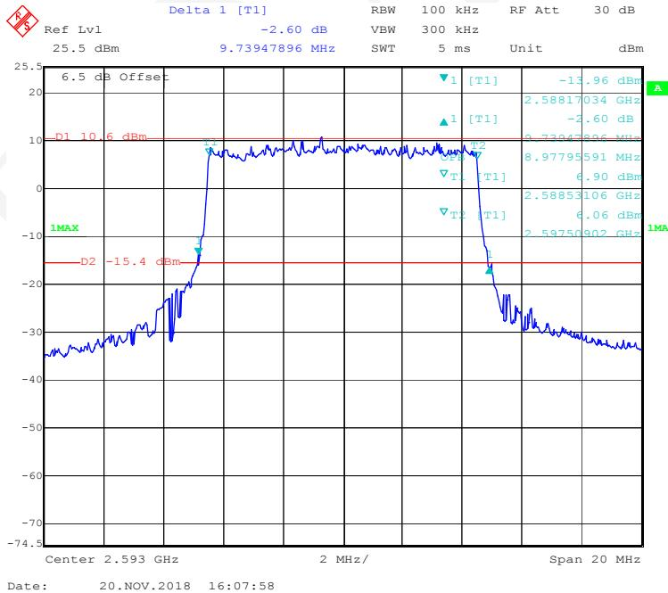
**16-QAM (15 MHz) - Middle channel**
