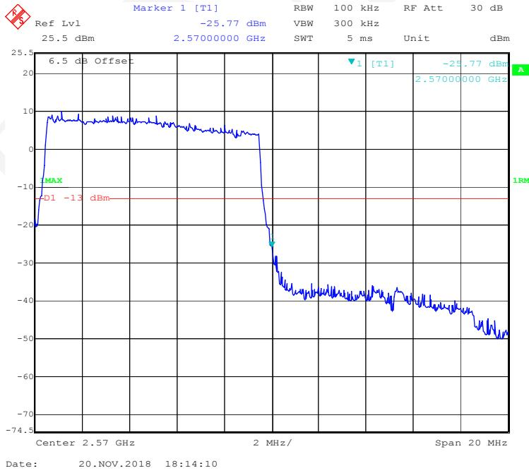
**16-QAM (15 MHz, FULL RB) - Left Band Edge**
