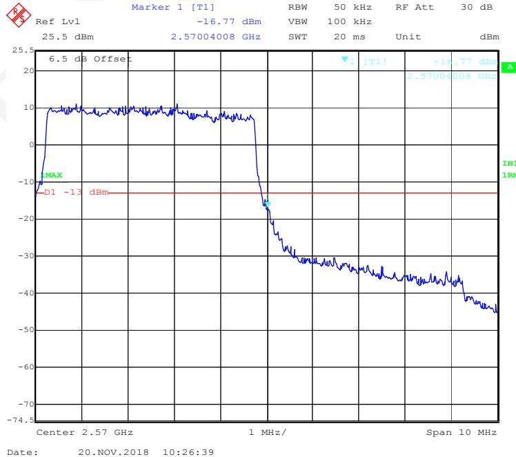
**QPSK (10 MHz, FULL RB) - Left Band Edge**
