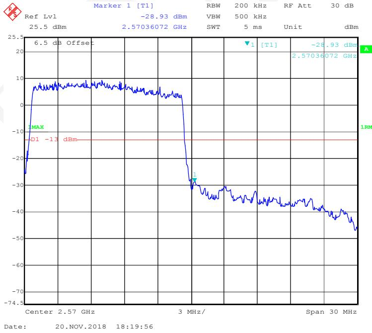
**QPSK (20 MHz, FULL RB) - Left Band Edge**
