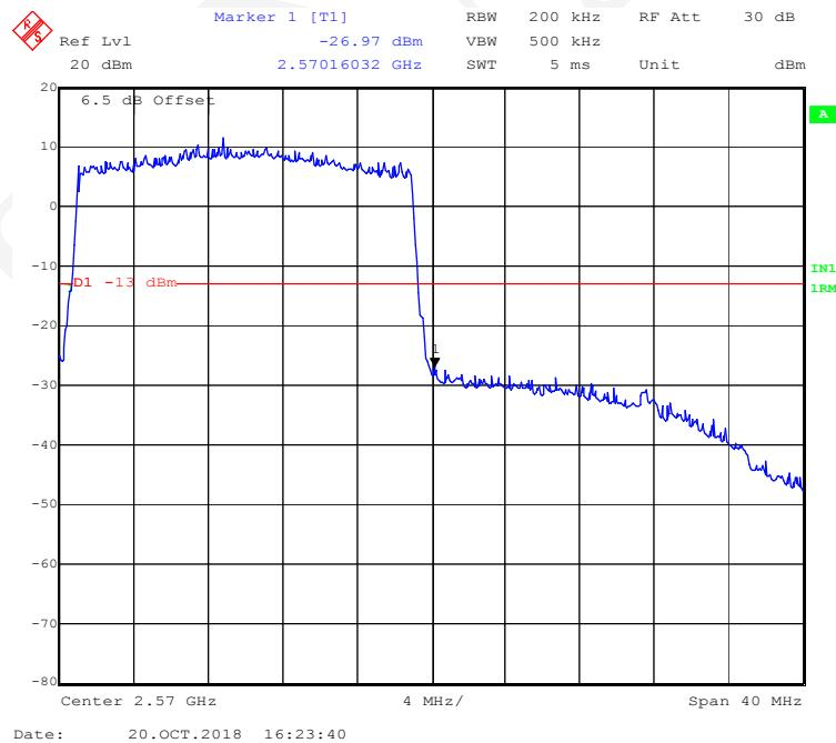
**16-QAM (5 MHz, FULL RB) - Left Band Edge**
