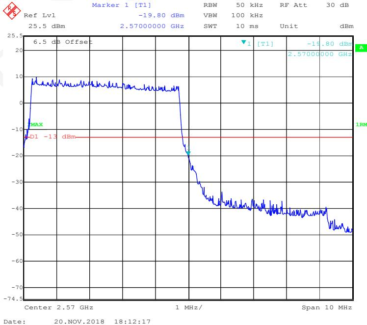
**QPSK (10 MHz, FULL RB) - Left Band Edge**
