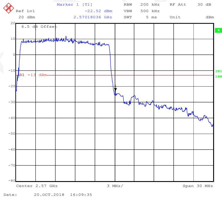
**QPSK (20 MHz, FULL RB) - Left Band Edge**
