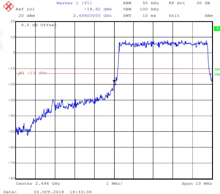
**QPSK (10 MHz, FULL RB) - Left Band Edge**
