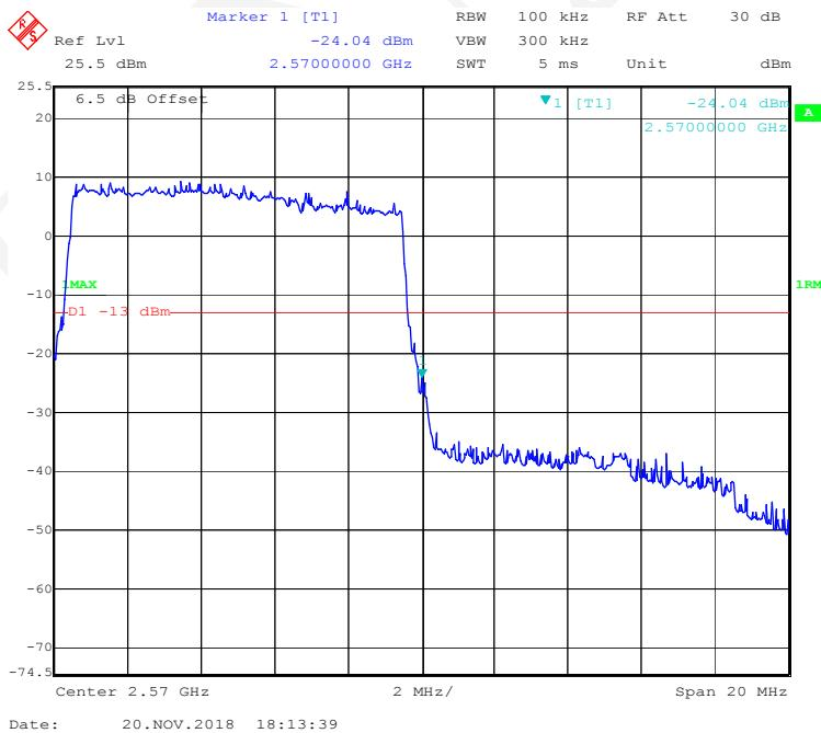
**QPSK (15 MHz, FULL RB) - Left Band Edge**
