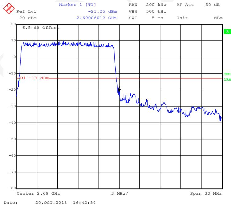
**QPSK (20MHz, FULL RB) - Left Band Edge**
