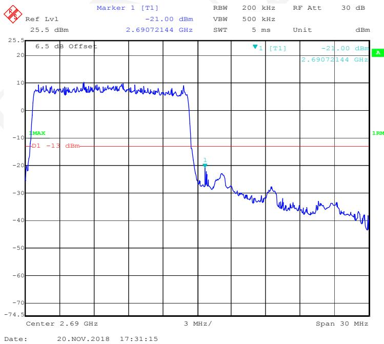
**QPSK (20MHz, FULL RB) - Left Band Edge**
