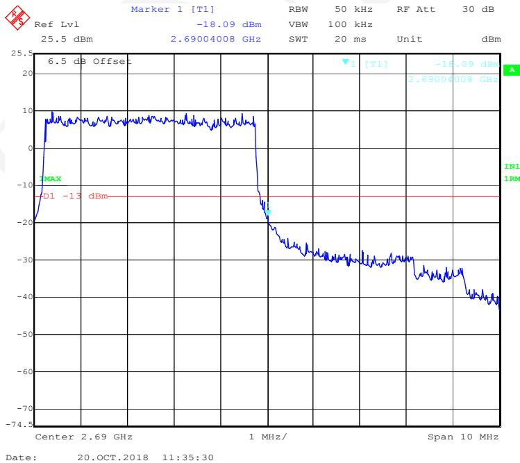
**16-QAM (10 MHz, FULL RB) - Left Band Edge**
