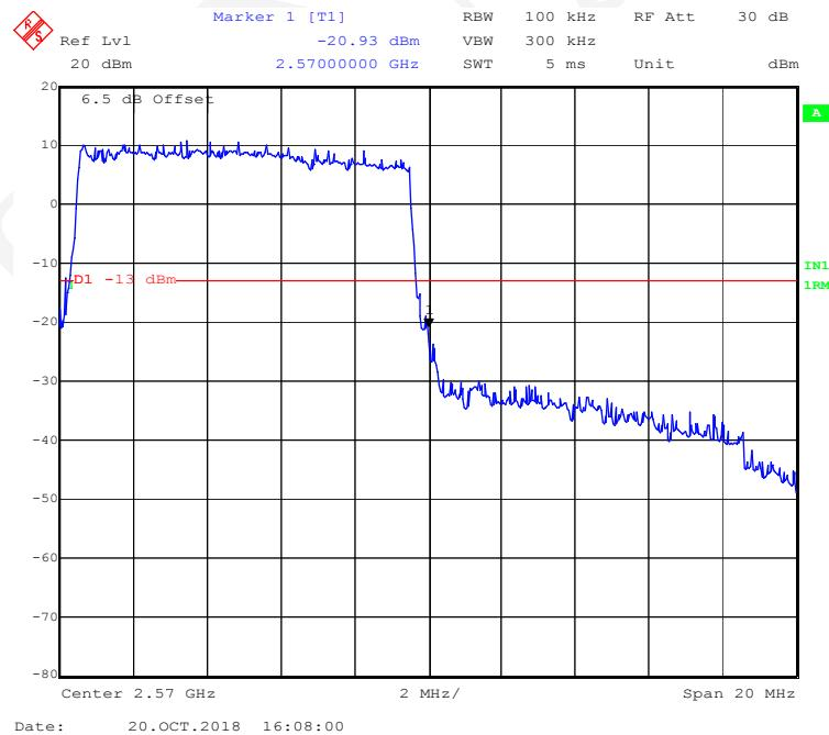
**16-QAM (15 MHz, FULL RB) - Left Band Edge**
