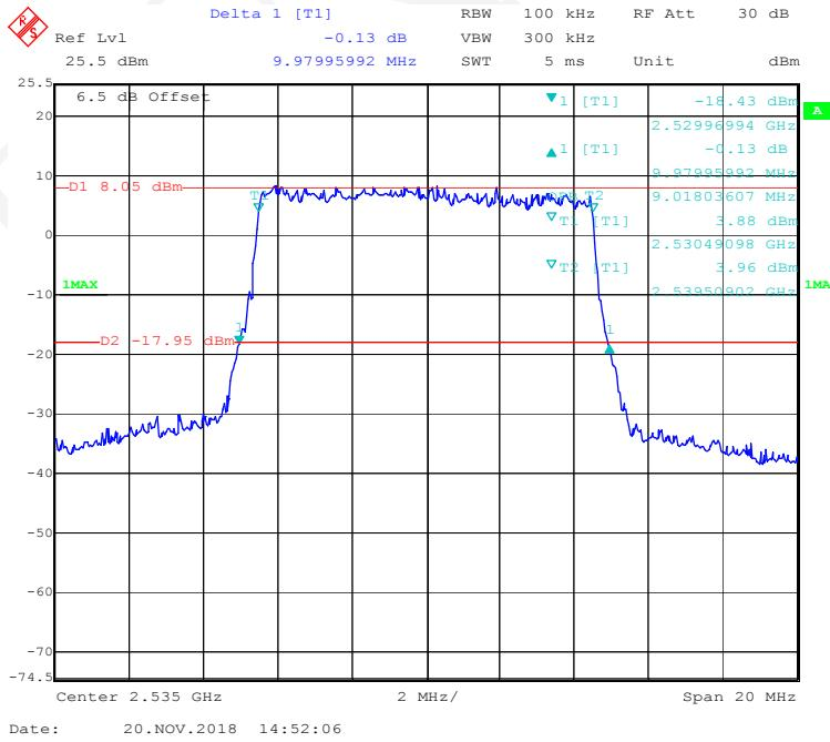
**QPSK (15MHz) - Middle channel**
