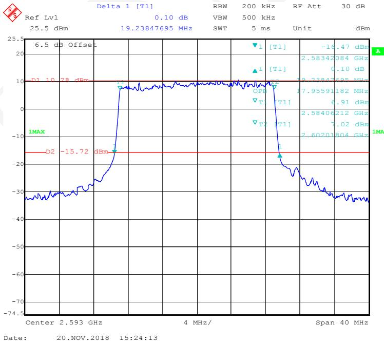
**16-QAM (5 MHz) - Middle channel**
