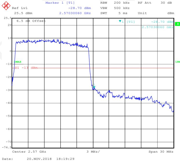
**16-QAM (20 MHz, FULL RB) - Left Band Edge**
