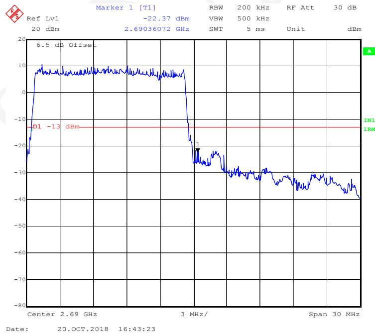
**16-QAM (20 MHz, FULL RB) - Left Band Edge**
