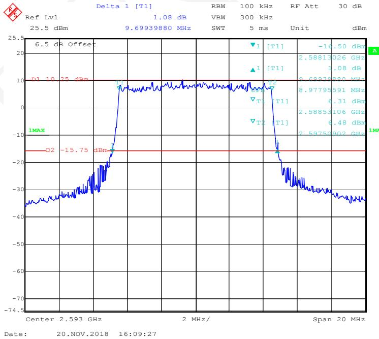
**QPSK (15 MHz) - Middle channel**
