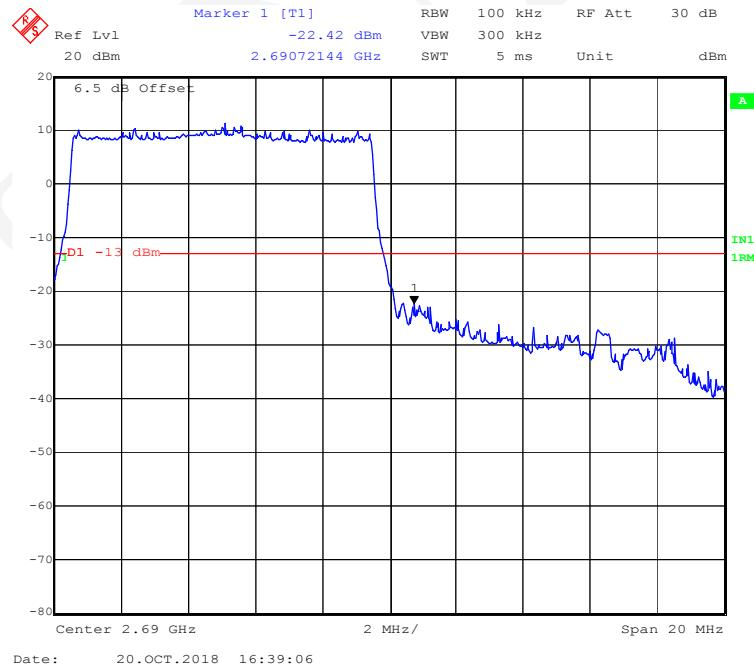
**16-QAM (15 MHz, FULL RB) - Left Band Edge**
