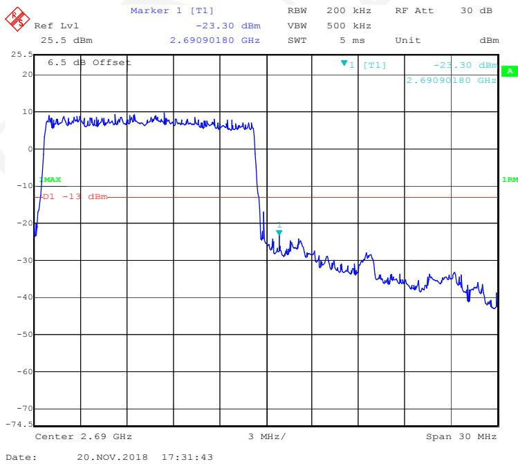
**16-QAM (20 MHz, FULL RB) - Left Band Edge**
