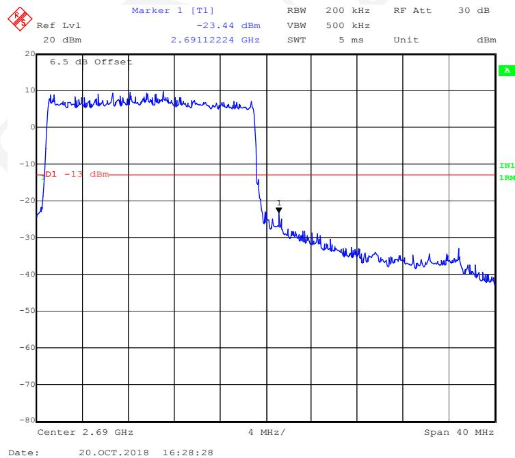
**16-QAM (5MHz, FULL RB) - Left Band Edge**
