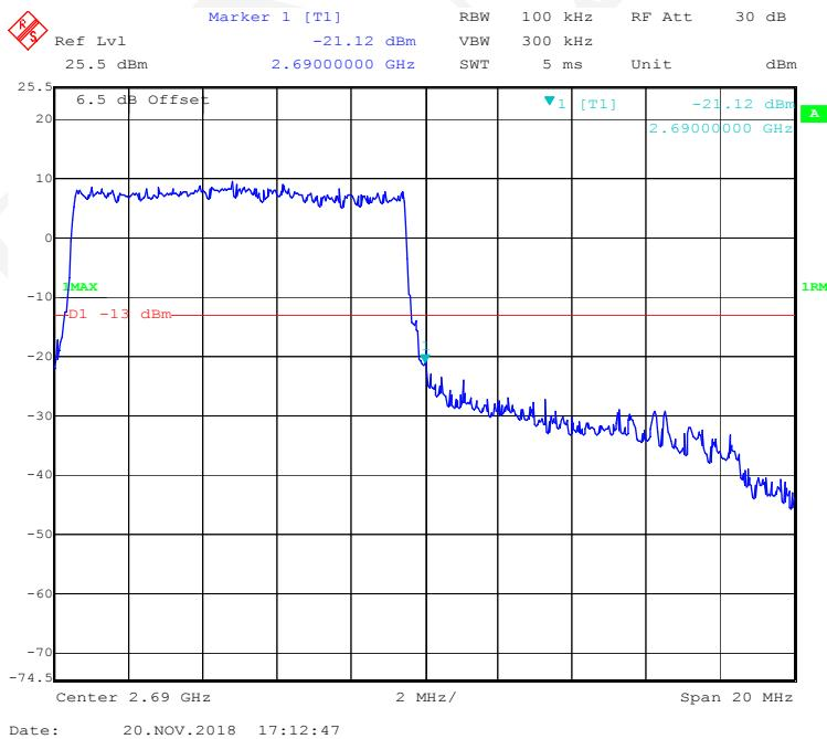
**QPSK (15MHz, FULL RB) - Left Band Edge**
