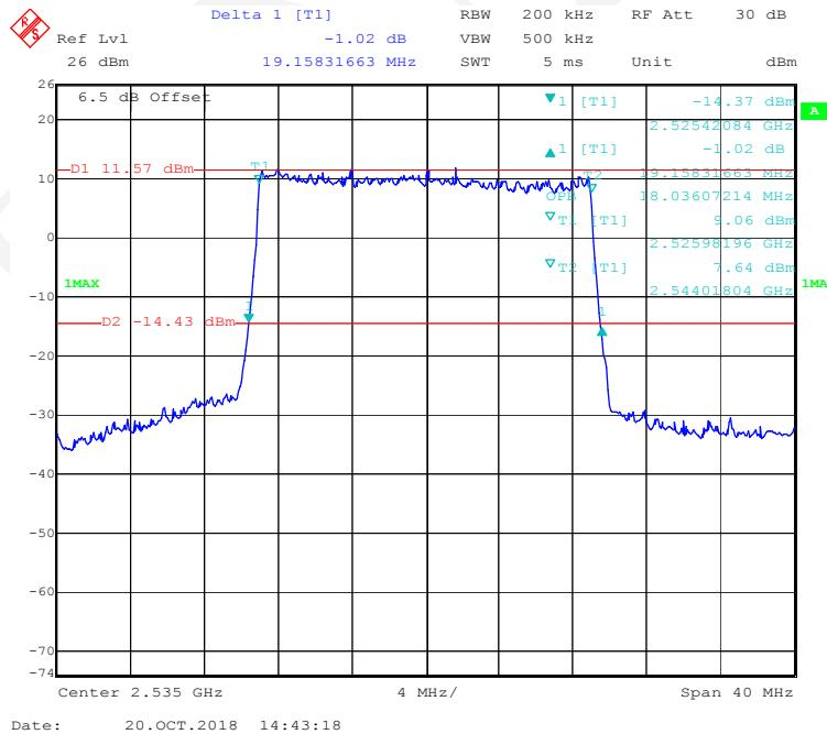
**16-QAM (5 MHz) - Middle channel**
