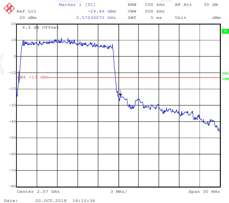
**16-QAM (20 MHz, FULL RB) - Left Band Edge**
