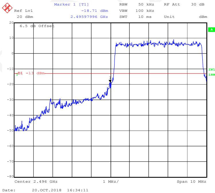
**16-QAM (10 MHz, FULL RB) - Left Band Edge**
