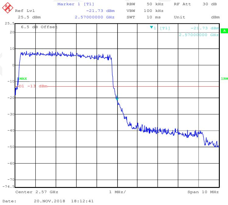
**16-QAM (10 MHz, FULL RB) - Left Band Edge**
