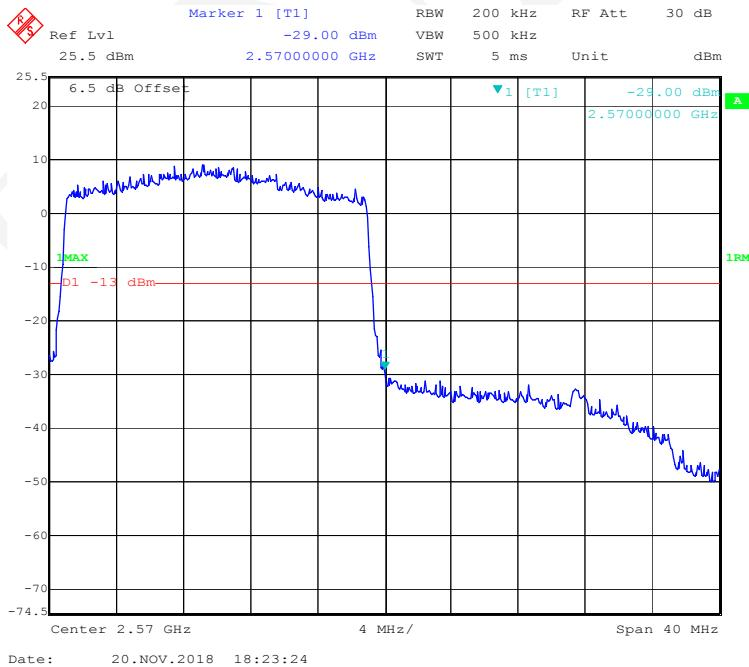
**16-QAM (5 MHz, FULL RB) - Left Band Edge**
