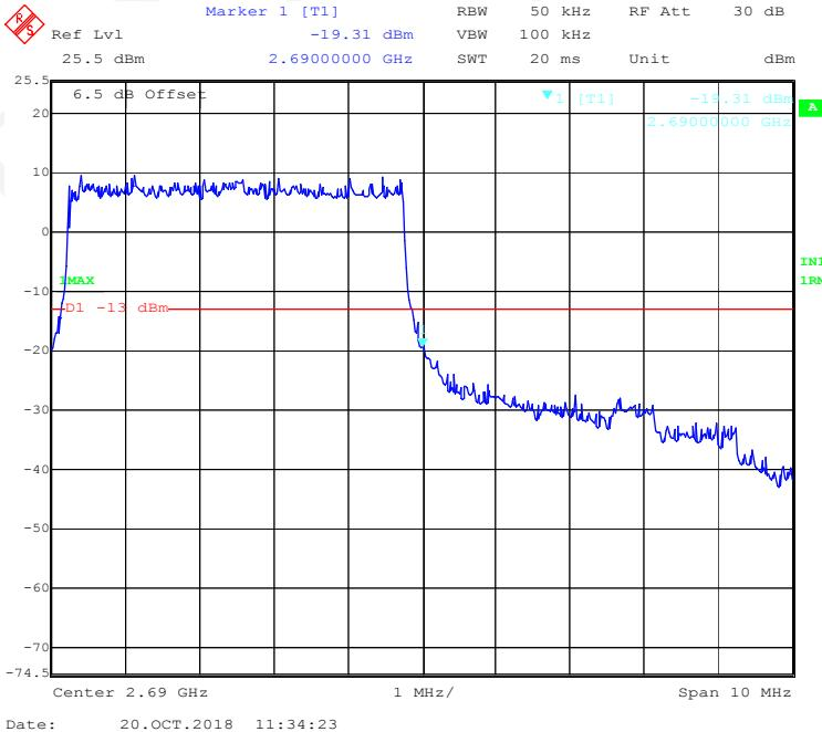
**QPSK (10 MHz, FULL RB) - Left Band Edge**
