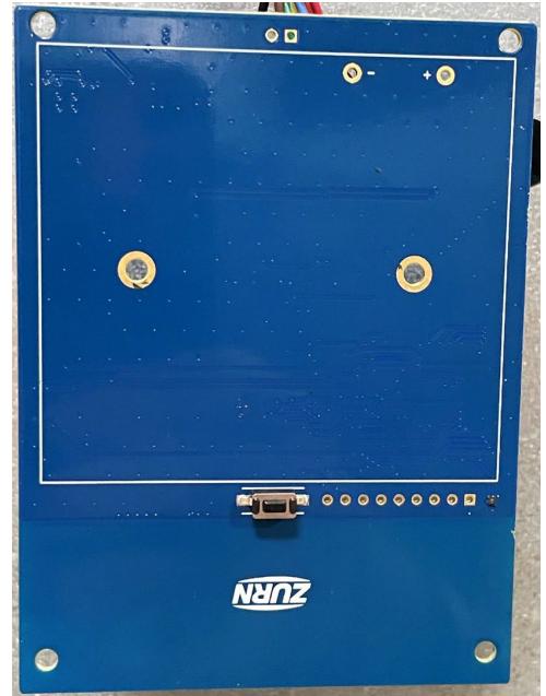
Endpoint (LoRa) Board w/trace antenna
