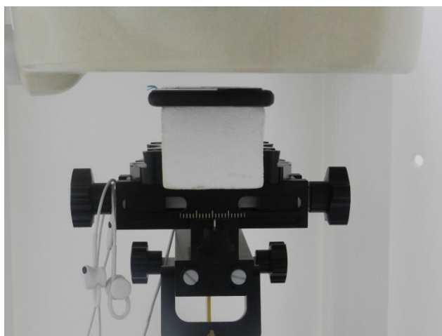
Back with headset, Test Separation 10 mm
