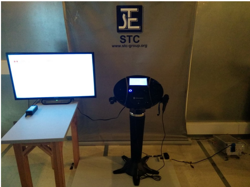
Measurement of Conducted Emission Test Set Up
