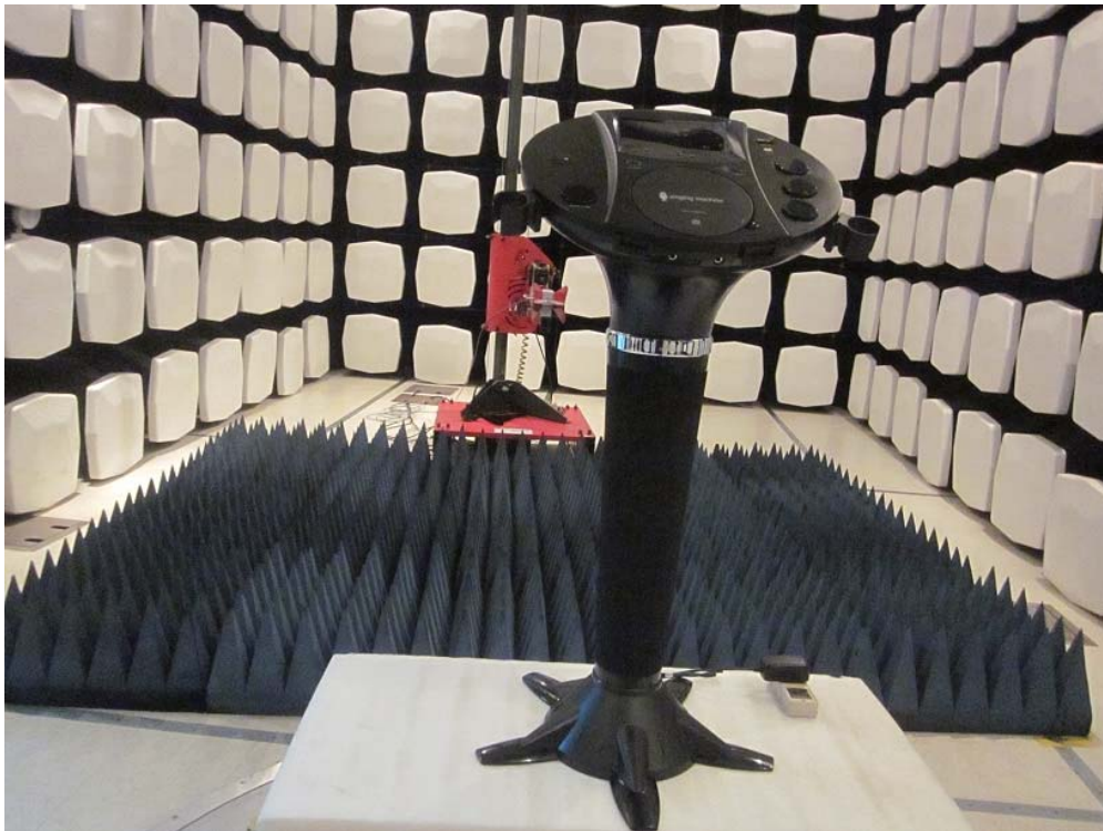
Measurement of Radiated Emission Test Set Up
