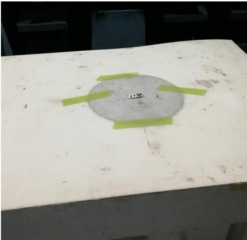
Figure 5: SAC Radiated Spurious Emissions – EUT w/o casing on turntable
