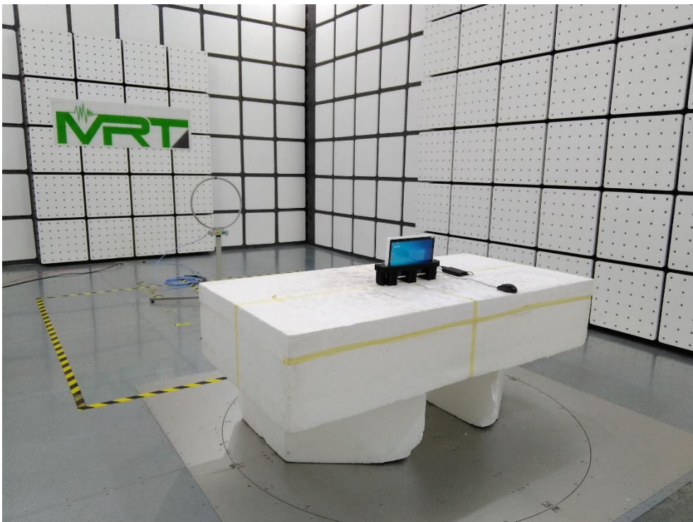
Description: Radiated Emission Test Setup for 9kHz~30MHz
