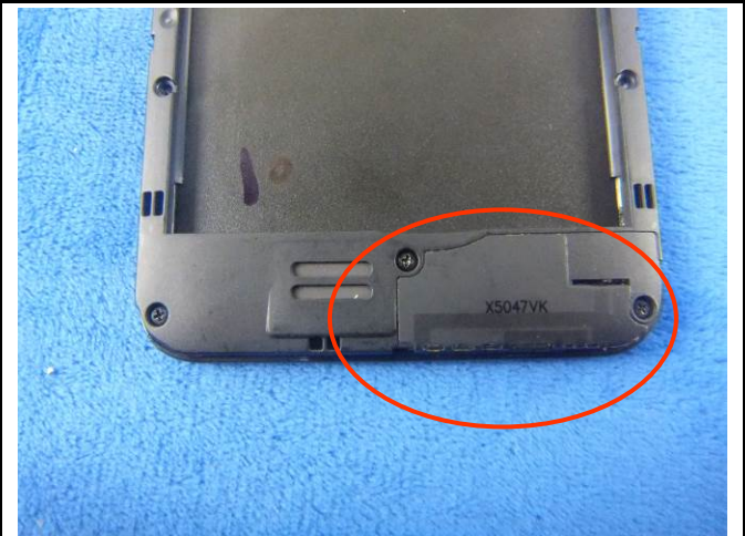
GSM/PCS/UMTS-FDD Antenna View
