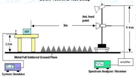
**Above 1GHz Test Setup**
