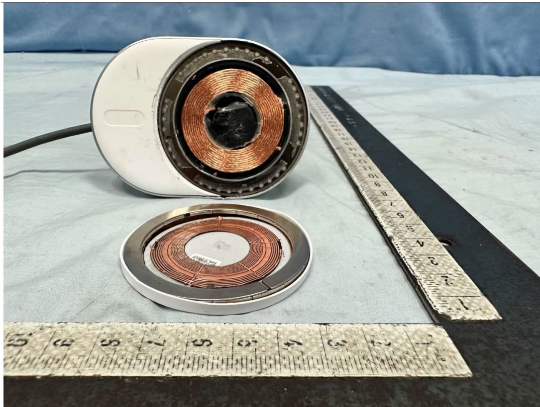
C223 Coil Antenna (MagSafe iPhones – 360 kHz) – Top View
