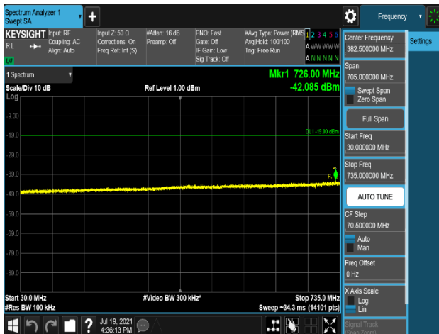
Plot 7-397. Conducted Spurious Emission Plot 30 MHz to 735 MHz (LTE_B13_5M+5M_2C_64QAM - Port 2)
