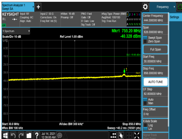
Plot 7-379. Conducted Spurious Emission Plot 30 MHz to 858 MHz (LTE_B5_10M+10M+2C_16QAM - Port 2)
