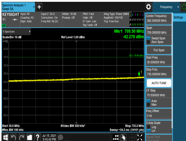
Plot 7-391. Conducted Spurious Emission Plot 30 MHz to 735 MHz (LTE_B13_10M_1C_16QAM - Port 2)
