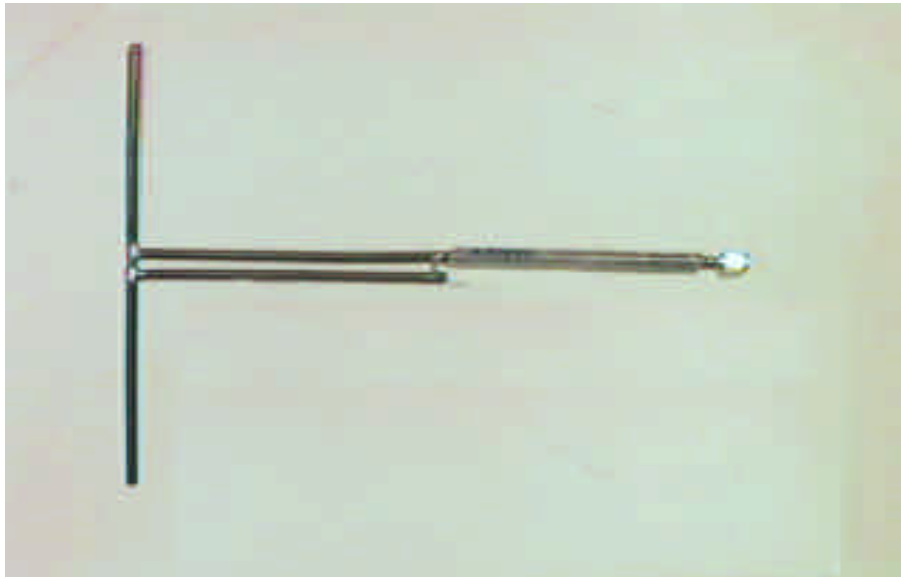
Reference Dipole Antenna Used for ERP Measurement
