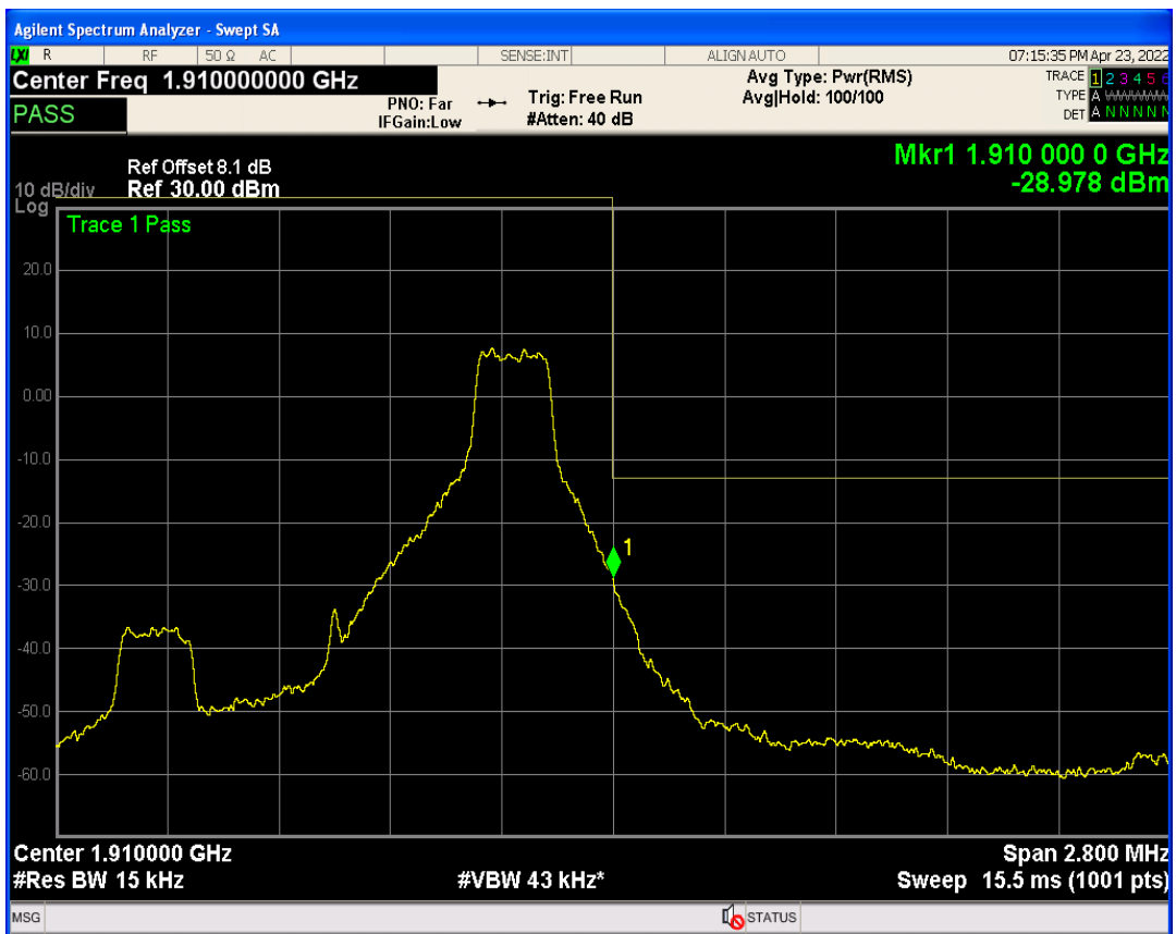
Band2 QPSK BW=1.4MHz Channel=19193 RB Size=6 Position=#0
