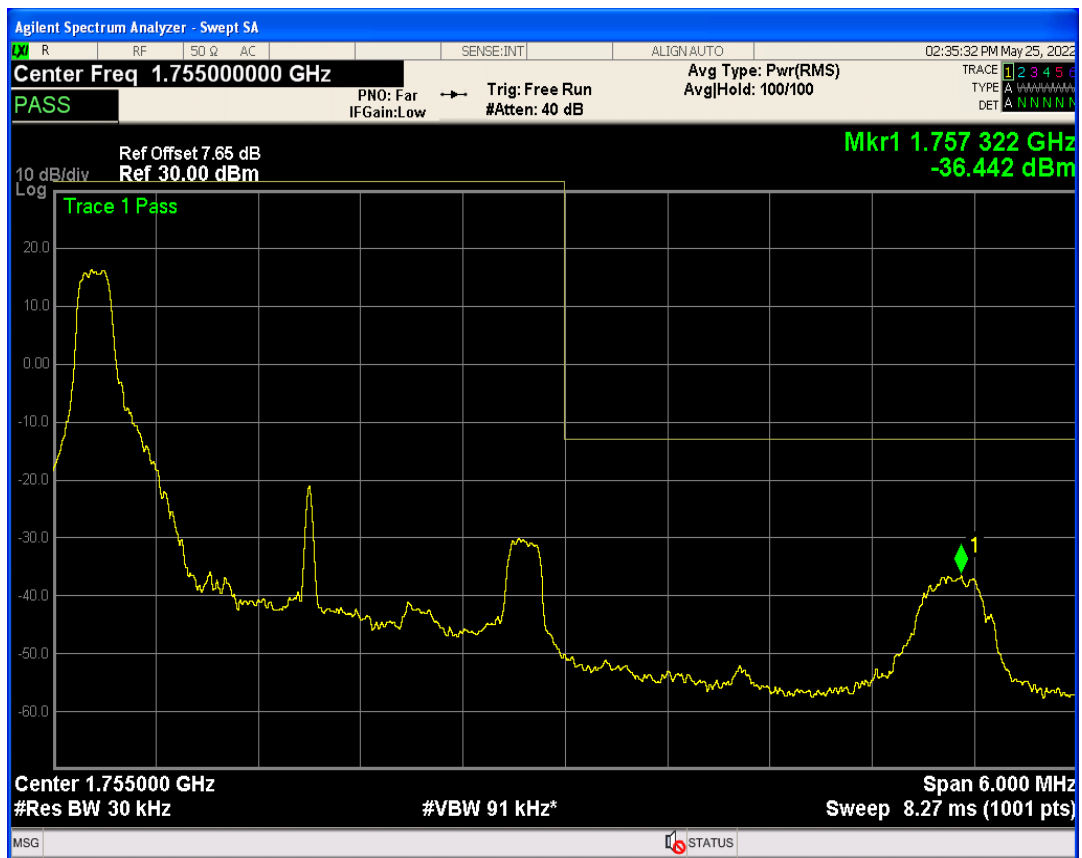
Band4 QAM16 BW=3MHz Channel=20385 RB Size=1 Position=#Max
