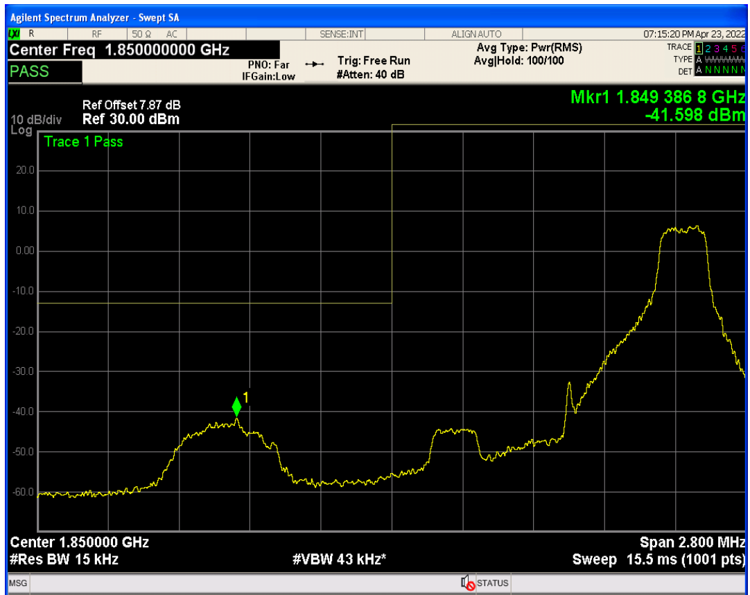
Band2 QAM16 BW=1.4MHz Channel=18607 RB Size=6 Position=#0
