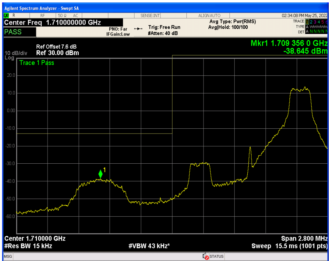
Band4 QAM16 BW=1.4MHz Channel=19957 RB Size=1 Position=#0
