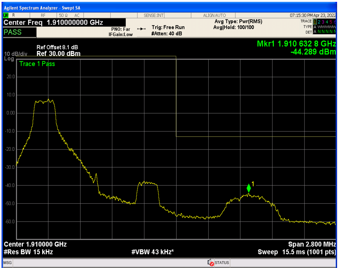
Band2 QPSK BW=1.4MHz Channel=19193 RB Size=1 Position=#Max
