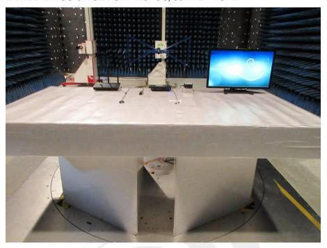
RADIATED EMISSION SET-UP PHOTOS, 1GHz ~ 25GHz
