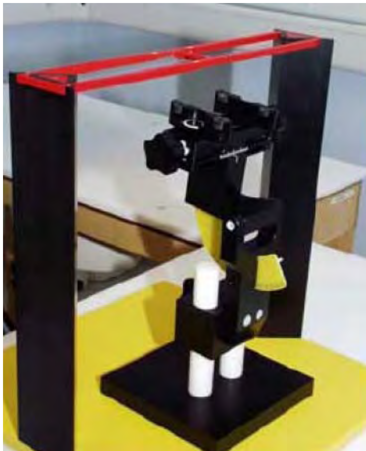
Figure 7 T-coil Phantom & Device Holder
