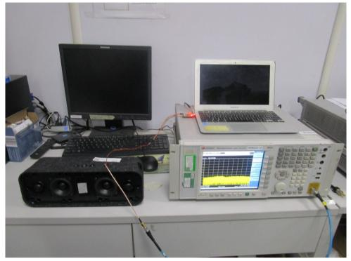
Conducted Emissions at AC Power Line (150kHz-30MHz)
