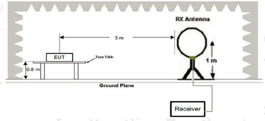
2. Radiated Emission Test-Up Frequency 30MHz~1GHz
