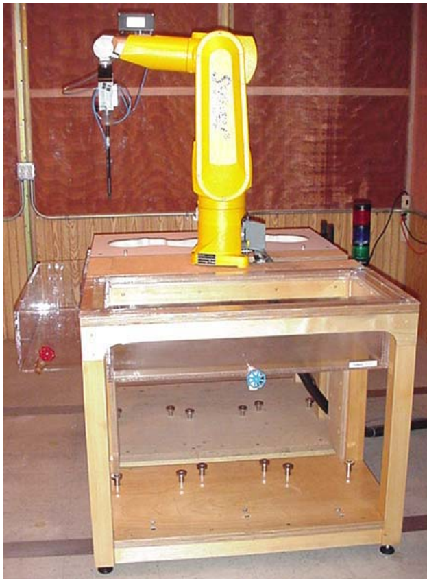
DASY4 SAR Measurement System with validation phantom
