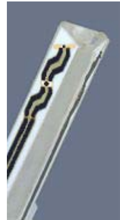
ET3DV6 E-Field Probe
