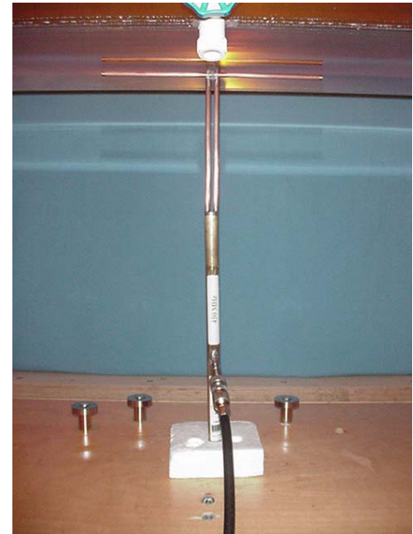
450 MHz Dipole Setup
