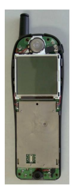
Handheld Portable MAIN Board (With Shield Case and Cover)
