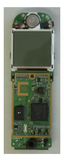
Handheld Portable MAIN Board (Front side, With Shield Cover Removed)
