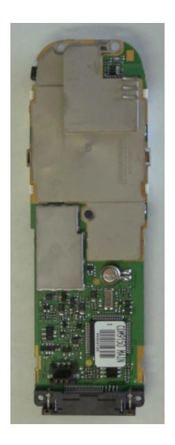
Handheld Portable MAIN Board (Back side, With shield cover)
