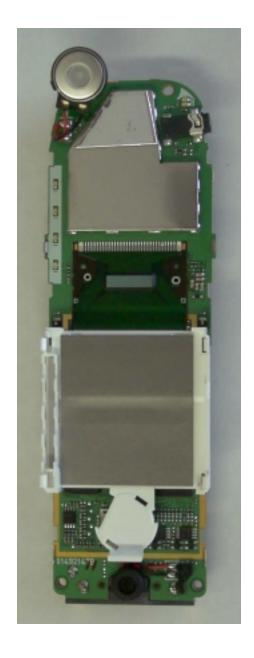
Handheld Portable MAIN Board (Front side, With Shield Cover and LCD holder Removed)
