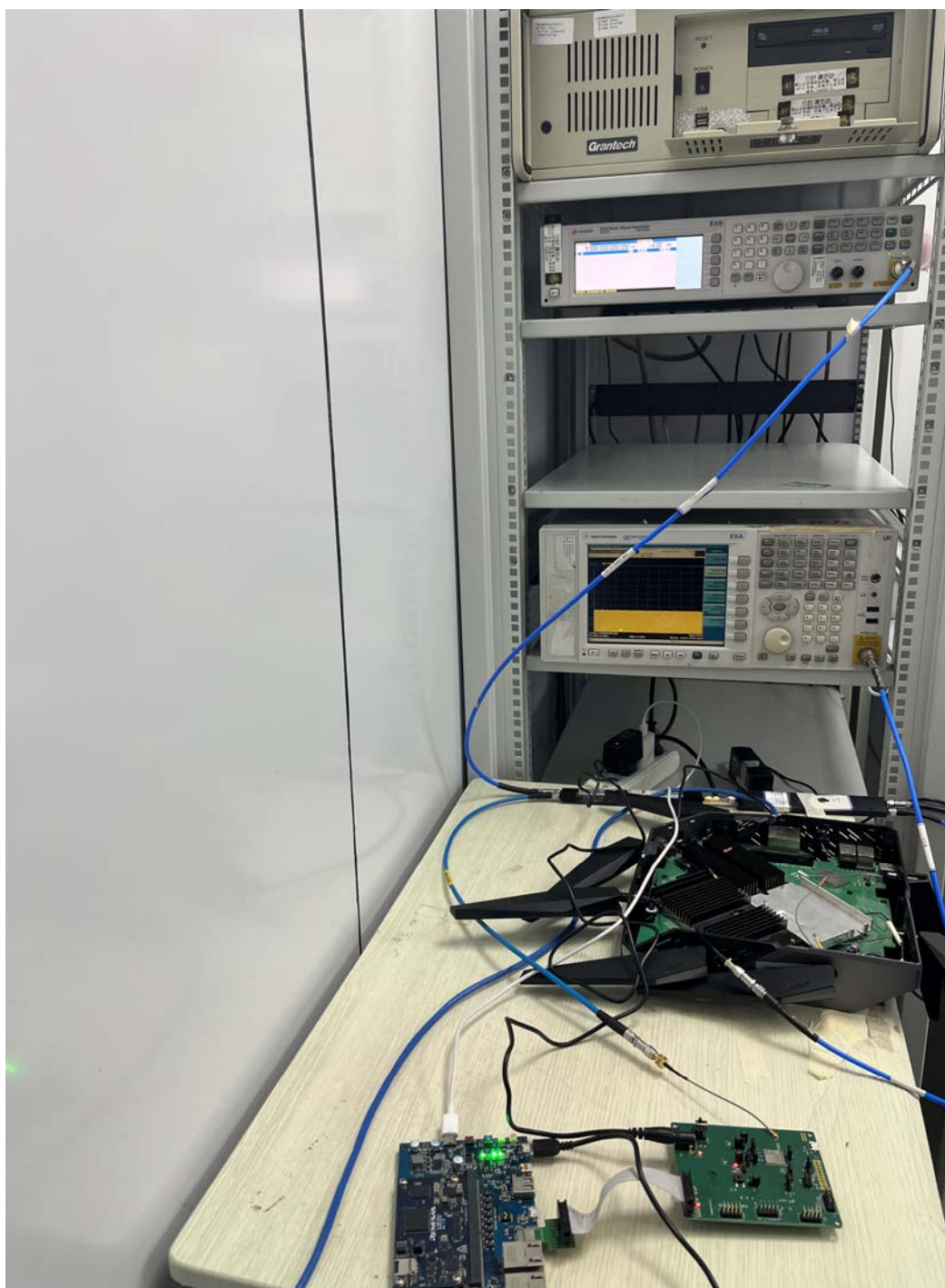
Picture 1 DFS Test Setup
