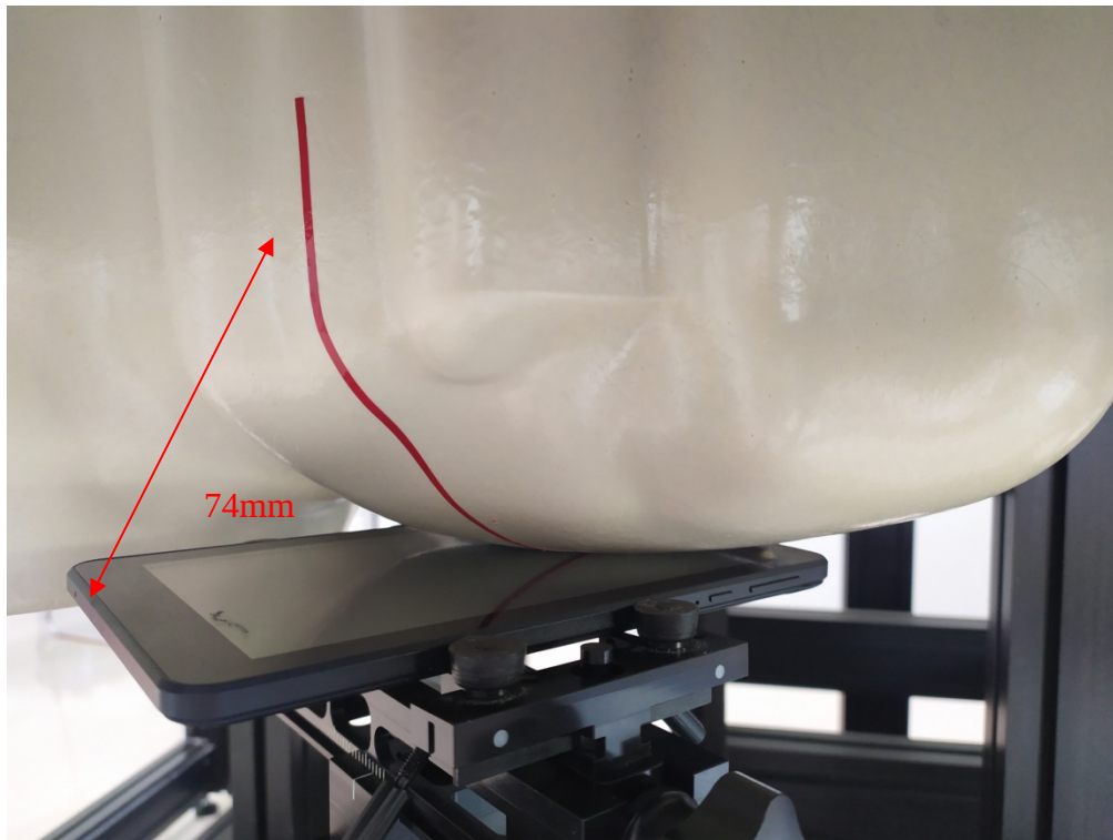
Head Left Cheek Setup Photo (0mm)
