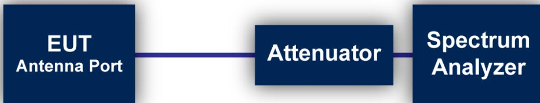
Figure 2: Direct Connection at the Antenna Port Test
