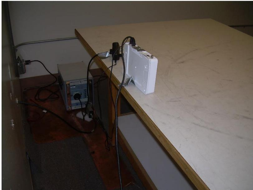
**Photograph 6: Back View Conducted Emissions Worst-Case Configuration**
