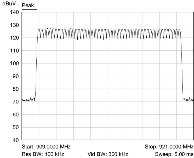
**Graph 12: Antenna 1 – Plot Showing All Channels Operate Within the Authorized Frequency Band**
