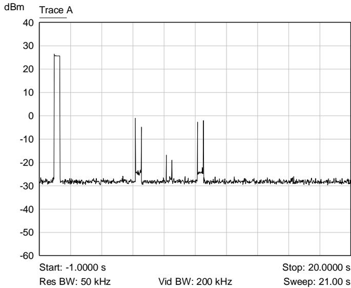
**Graph 6: Timing Plot Showing Channel Hits**
