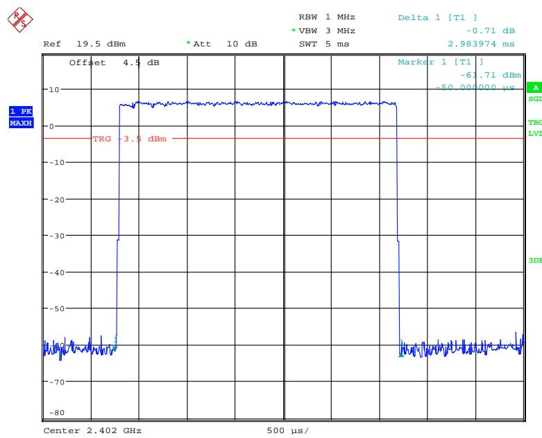
**Pulse time, Middle Channel, 2DH5**
