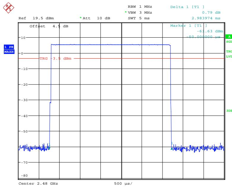
**EDR ( $\pi/4$ -DQPSK):****Pulse time, Low Channel, 2DH1**
